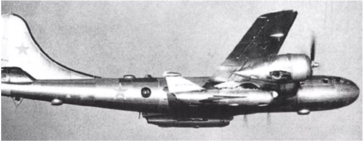
An extra challenge to the defence came with the introduction of air-launched stand-off missiles, initially referred to as 'powered bombs'. This shows a Tu-4K carrying two AS-1 'Kennel'.
