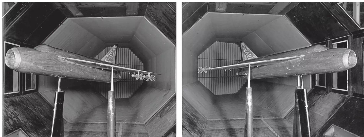
Two views of the P1A model in the 9 x 7ft wind tunnel during tests to find suitable locations for carrying extra missiles.
