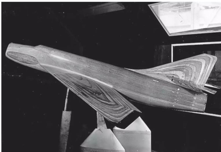
Two views of the P1 model in the English Electric 9 x 7ft wind tunnel, September 5, 1949. Crucial to finding the best layout, it allowed testing of different tailplane locations and was later modified to allow the wing to be repositioned. It is currently on display in the Heritage Department at Warton Aerodrome.
