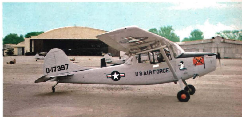
Above, a Cessna O-1F of the type widely used for Forward Air Controller duties by the USAF; this one has an M.60 machine gun under each wing. Below, a loudspeaker is mounted on the port side of this Helio U-10, used primarily in the psychological warfare campaign.
