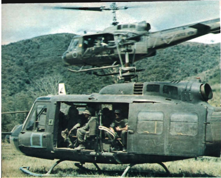
Bell UH-1 helicopters are widely used in Vietnam in a number of different roles. Illustrated here are US Army UH-1D "Slicks", the standard troop-carrying version of the Iroquois.
