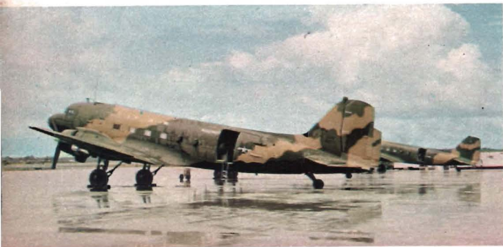
Above, a newly painted A-1 of the VNAF's 518 Tactical Fighter Squadron. Below, AC-47As, the highly successful "Puff-Ships" or "Magic Dragons" which can let loose 18,000 rounds per minute from three General Electric Miniguns.
