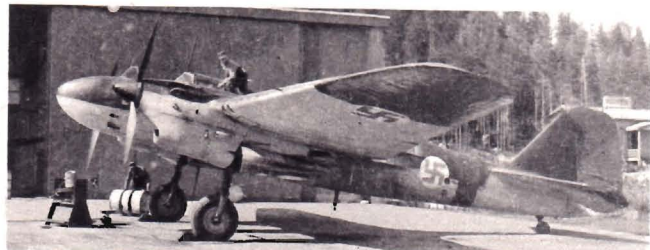
Above, a number of SB-2bis bombers were converted for the pilot training role, and this captured example (SB-5) is seen in service with the Finnish Air Force. Left, this late production example of the SB-2bis serving with the VVS early in 1942 was fitted with one of the several types of dorsal turret eventually fitted to this type, and had a more elaborate ventral gun position.
