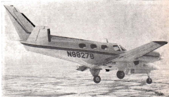
First flown on December 29, 1966, the Beechcraft Duke is a six-seat twin-engine addition to the Beech range. Powered by 380 hp turbo-supercharged Lycoming engines, the Duke has a gross weight of 6,400 lb (2,900 kg) and deliveries will begin next October.
