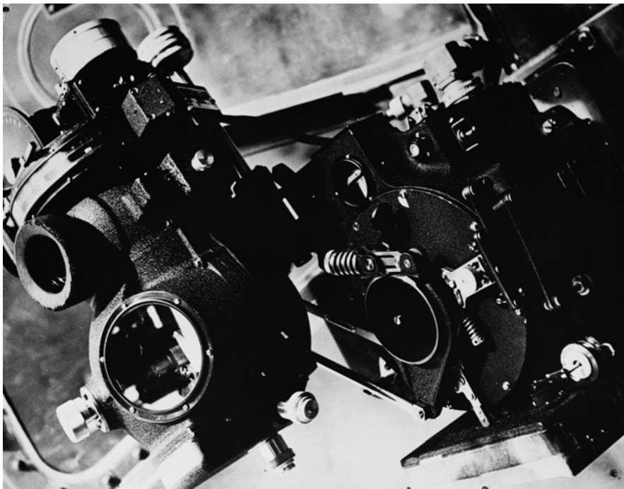
Developed during World War II, the Norden bombsight enabled B-29 bombardiers to aim their weapons visually with great precision. (© Corbis via Getty Images)
