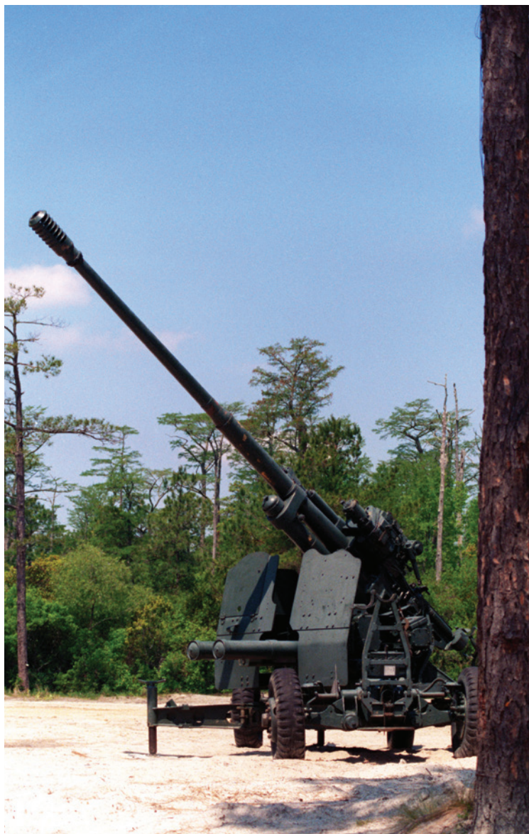
A Soviet 100mm KS-19 anti-aircraft gun. In theory, these weapons could reach up to 40,000ft; they presented a considerable threat to propeller-driven bombers like the B-29. (US National Archive)
