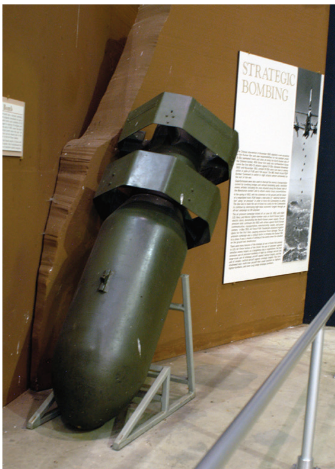
The 1,000lb VB-3 RANge and AZimuy ONLY (RAZON) radio-guided bomb proved the viability of precision-guided munitions in combat, but also highlighted some of the practical problems in using them. (NMUSAF)
