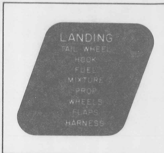
Figure 2-3. Landing Check List
