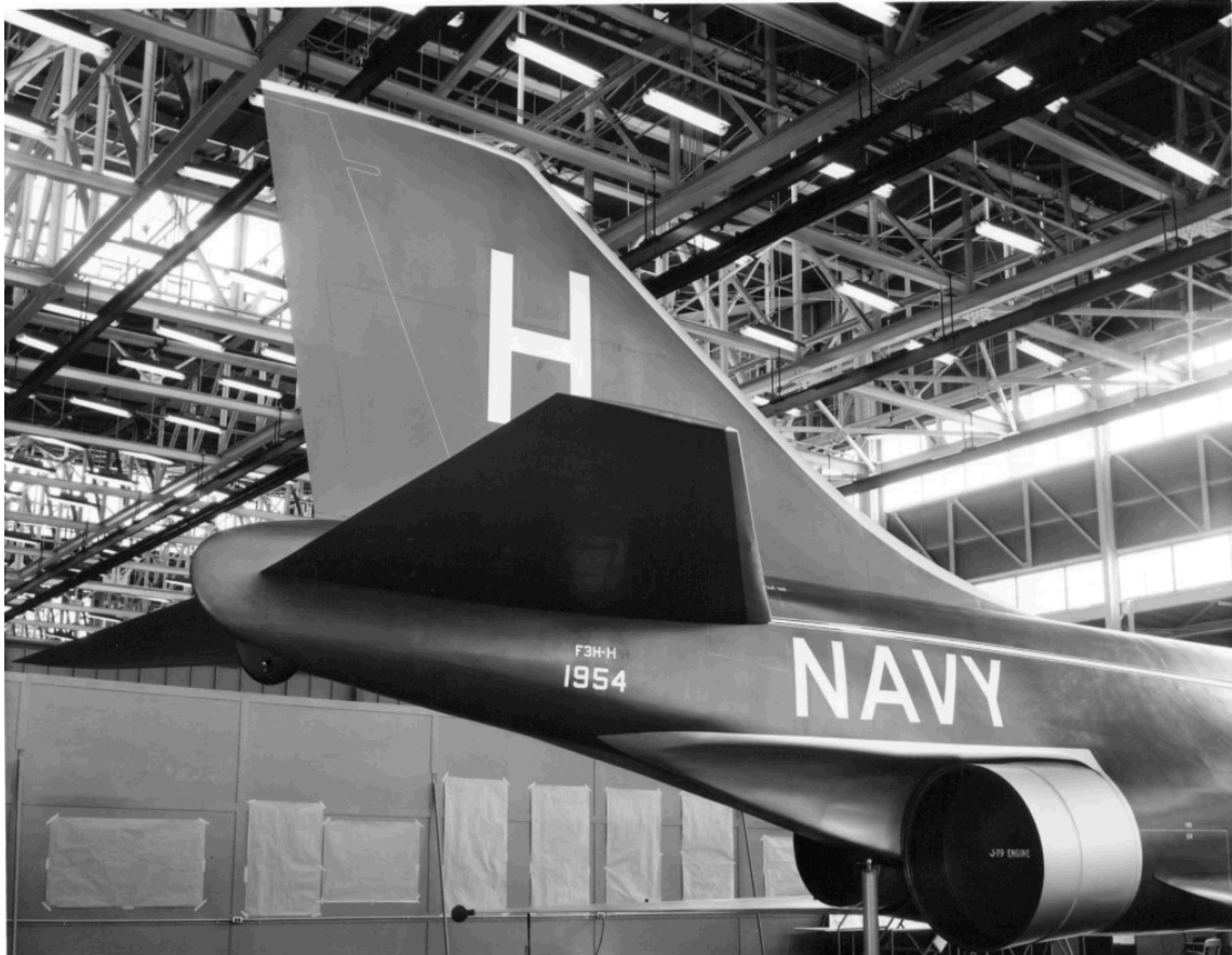
TAIL SECTION OF THE F3H-G MOCKUP SHOWING THE TWO DIFFERENT ENGINE SIZES- THE J79 WAS ON THE RIGHT SIDE, THE J65 WAS ON THE LEFT SIDE. (WIKIPEDIA)
