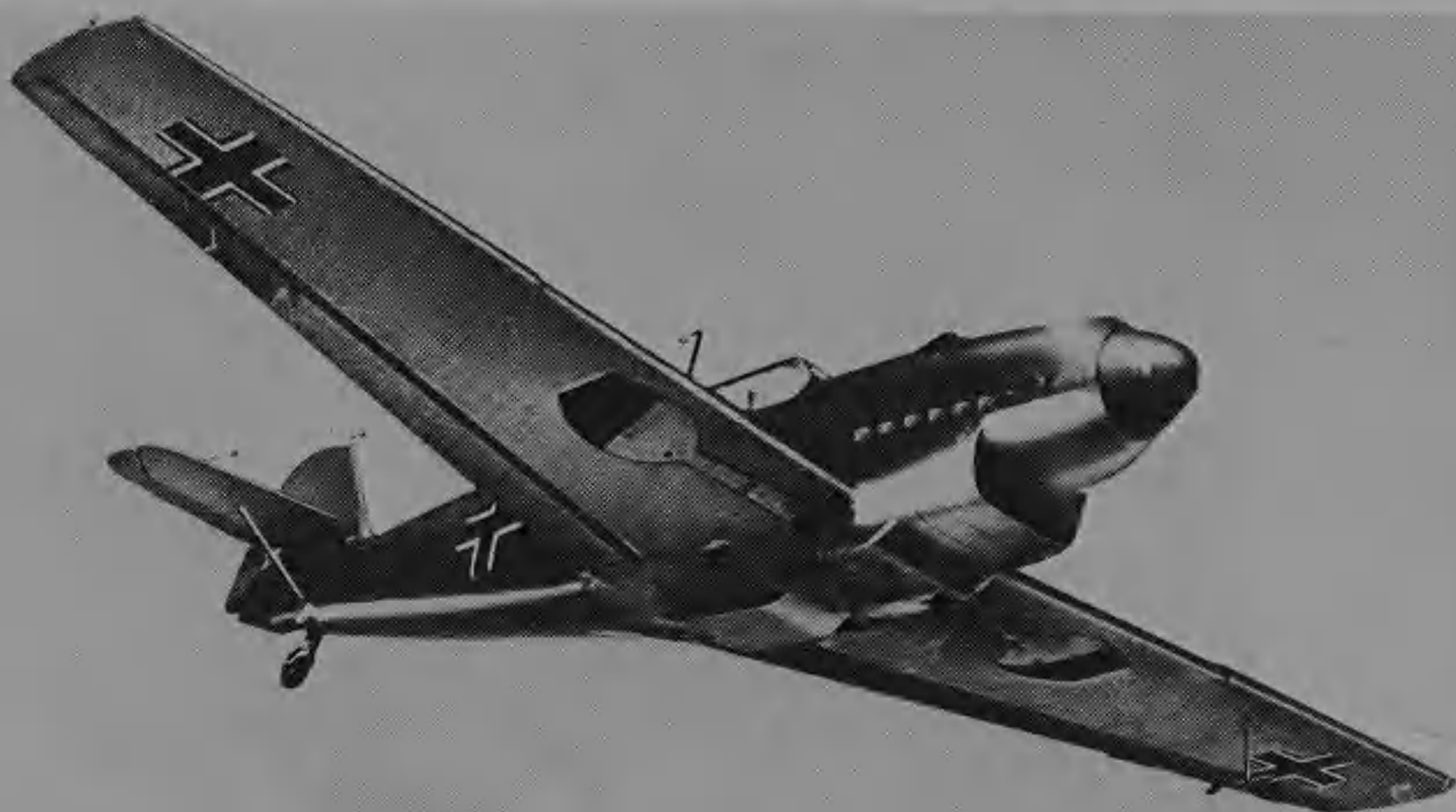
Below: The Messerschmitt Me 109, most widely used German fighter of the war. It was in the same class and had a similar record to the Spitfire. More than 33,000 were built and fought on all battle fronts where the Luftwaffe saw action. Its 1,100 hp gave it a top speed of 354 mph, a ceiling of 36,000 ft, range of 410 miles and its armament was two cannon and two machine-guns.
