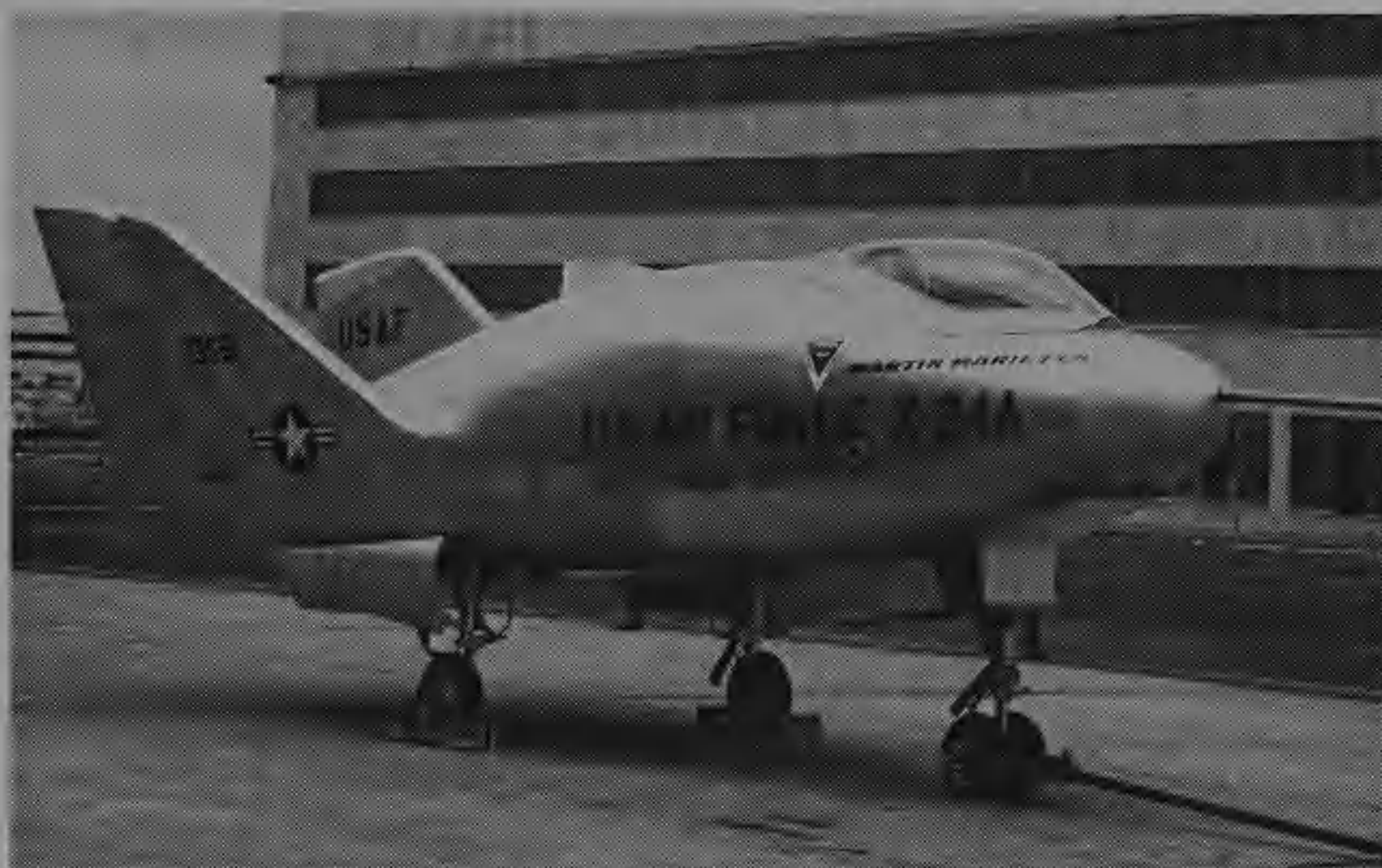
Above: Towards cheap space travel: the X-24 manned lifting body. Craft like these will, in the not too distant future, be boosted into space and be able to return to earth like an ordinary aircraft. The technique means that they can be used over and over again, cutting out the wasteful multi-stage rocket of today.
