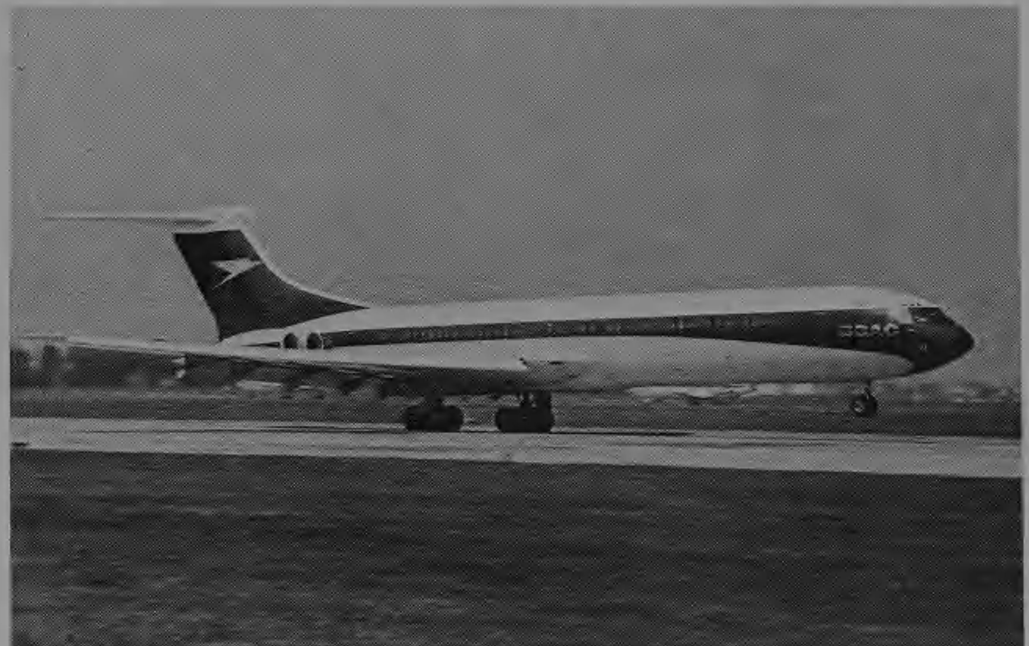
Right: The British answer to the big American jets was the VC-10 with its four engines grouped at the rear and a T-tail. But the completely "clean" wings had to be made thick enough to stop flutter and this makes an airliner heavier.
