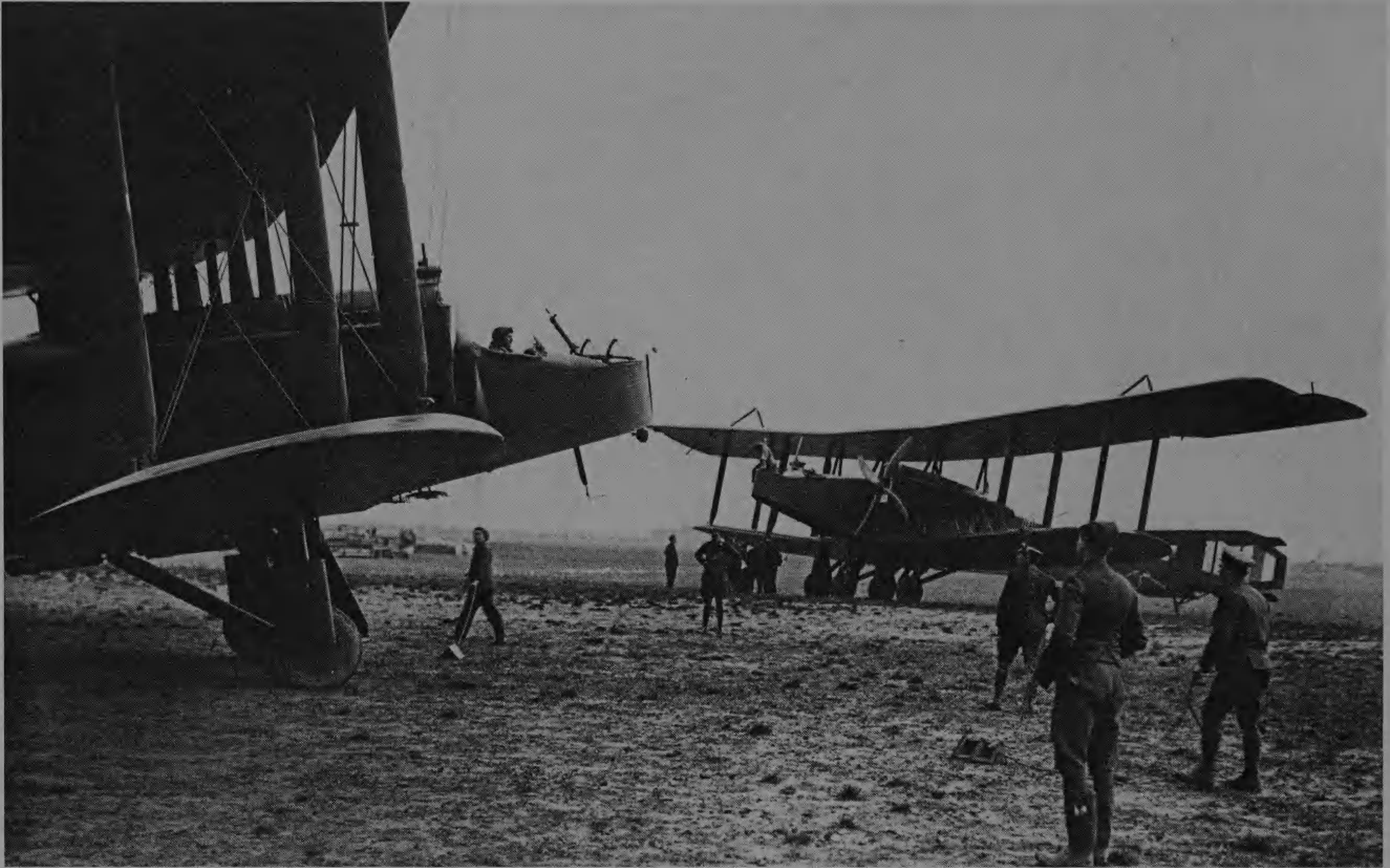
Above: Bombers begin to emerge: Handley Page O/400s prepare for a raid at a Royal Naval Air Service airfield near Dunkirk on April 20, 1918. The O/400s operated mainly at night and their twin 360 hp engines gave them a speed of 98 mph and a range of 370 miles. Armament was 1,800 lb of bombs and up to five machine-guns.
