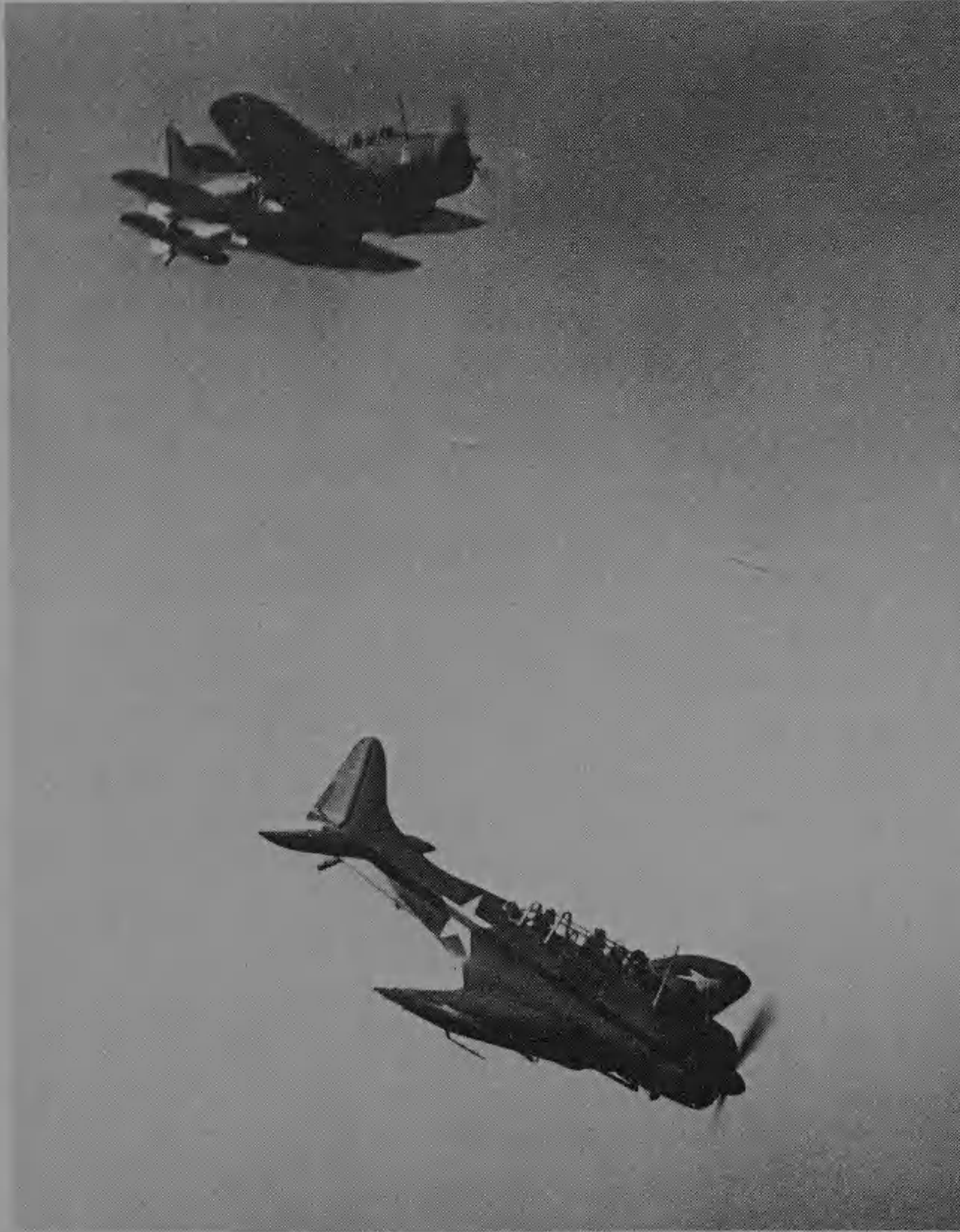
Above: A Douglas Dauntless dive bomber zooms into the attack during an action in the Pacific. At the Battle of Midway Island Dauntlesses sank three Japanese carriers and helped to destroy a fourth. The planes were two-seaters with a single 1,000 hp engine, a top speed of 250 mph and a range of 1,345 miles.
