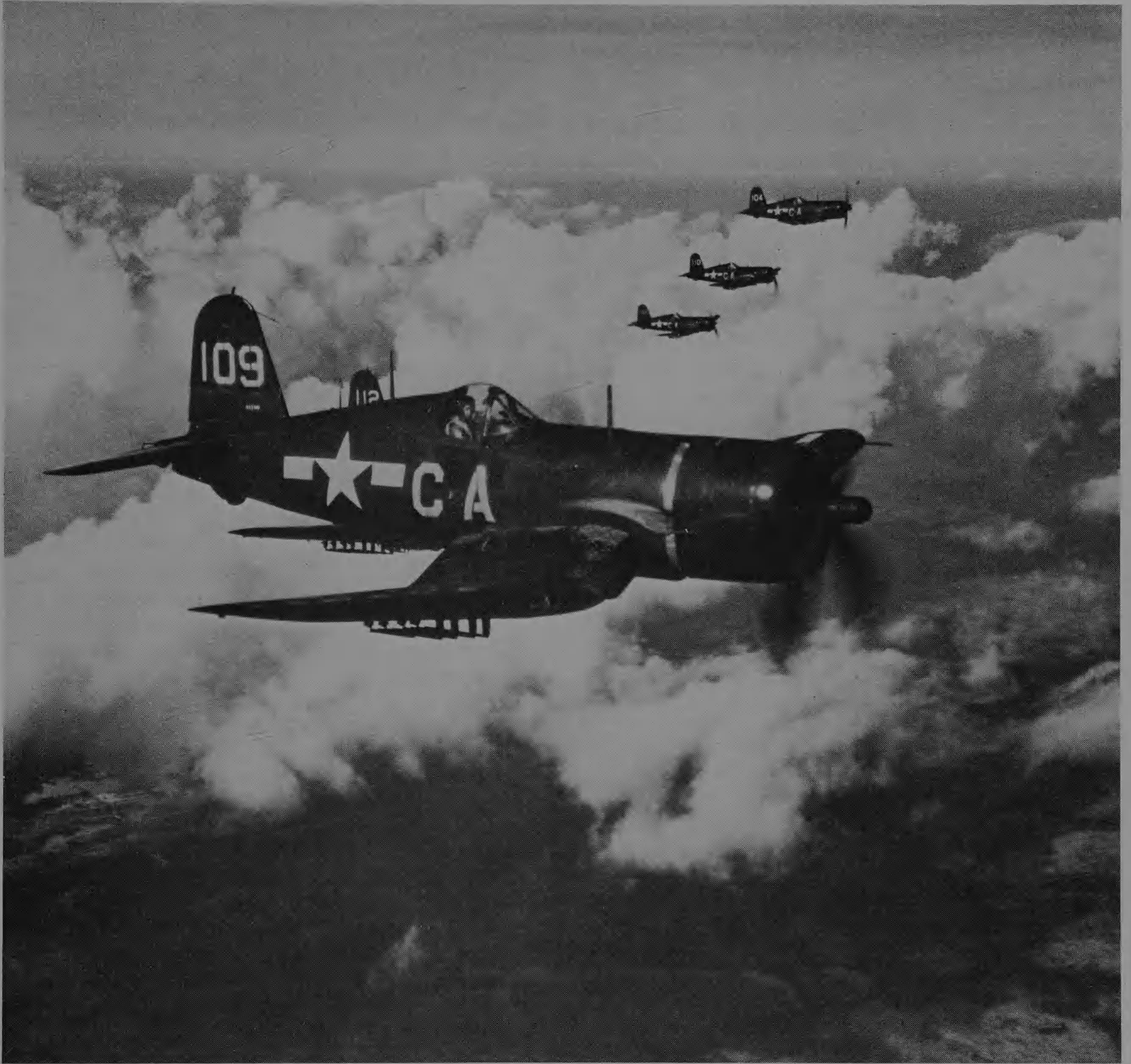
The Vought F4U Corsair was regarded by many Japanese pilots as the best Allied fighter. It first went into action in 1943 and was capable of over 400 mph. An unusual feature of the aircraft was its "kinked" wings.
