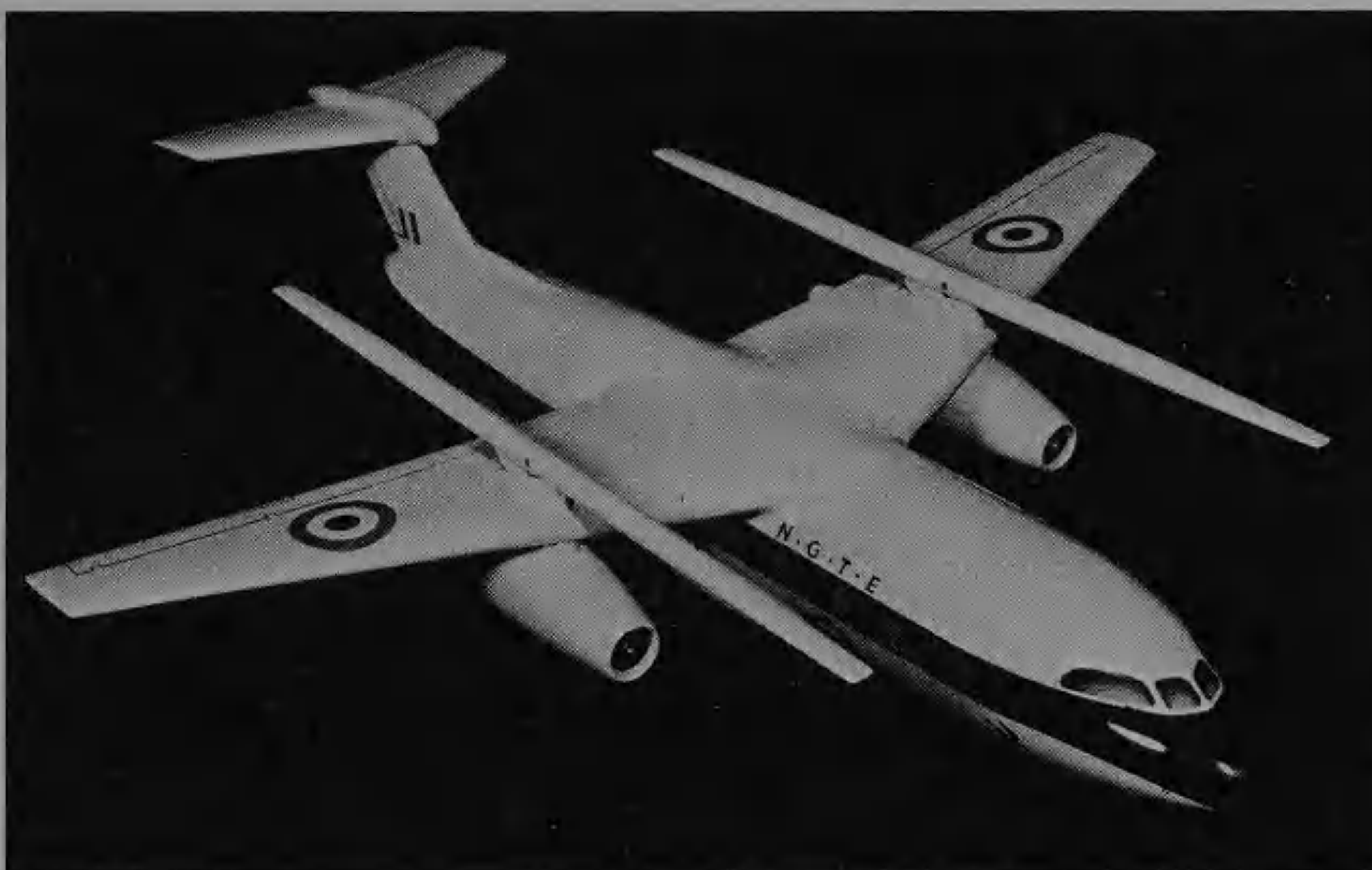
Foot of page: Hot cycle: The Hughes idea for a helibus which has dual-purpose wings. They rotate to give low speed and hovering flight and are stopped when the aircraft is cruising.
