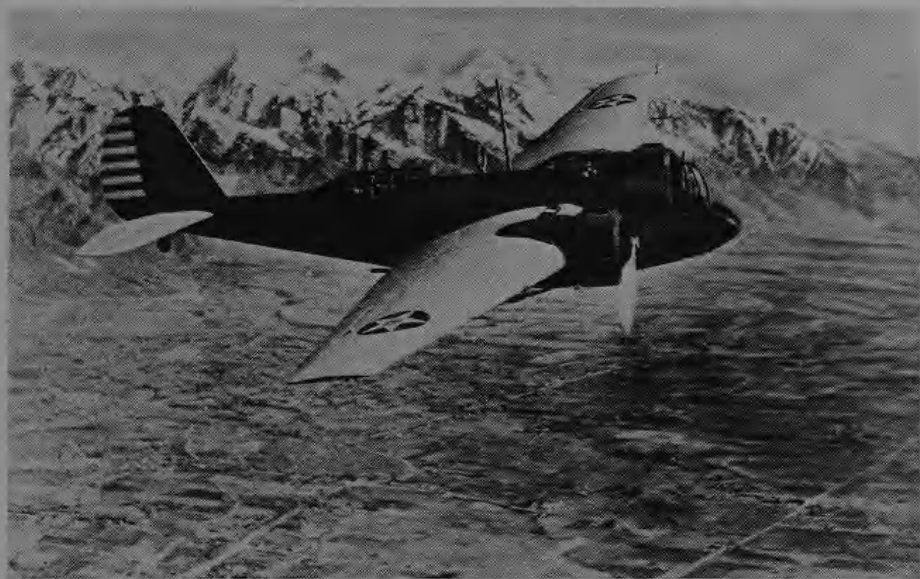
Above: The plane the US Army chose instead of the Boeing, the Martin B-10. This is the B-10 B, the largest model of the series. Its wing-span was 70 ft, length 45 ft, speed 212 mph and its engines were two Wright R-1820-33 of 740 hp.
