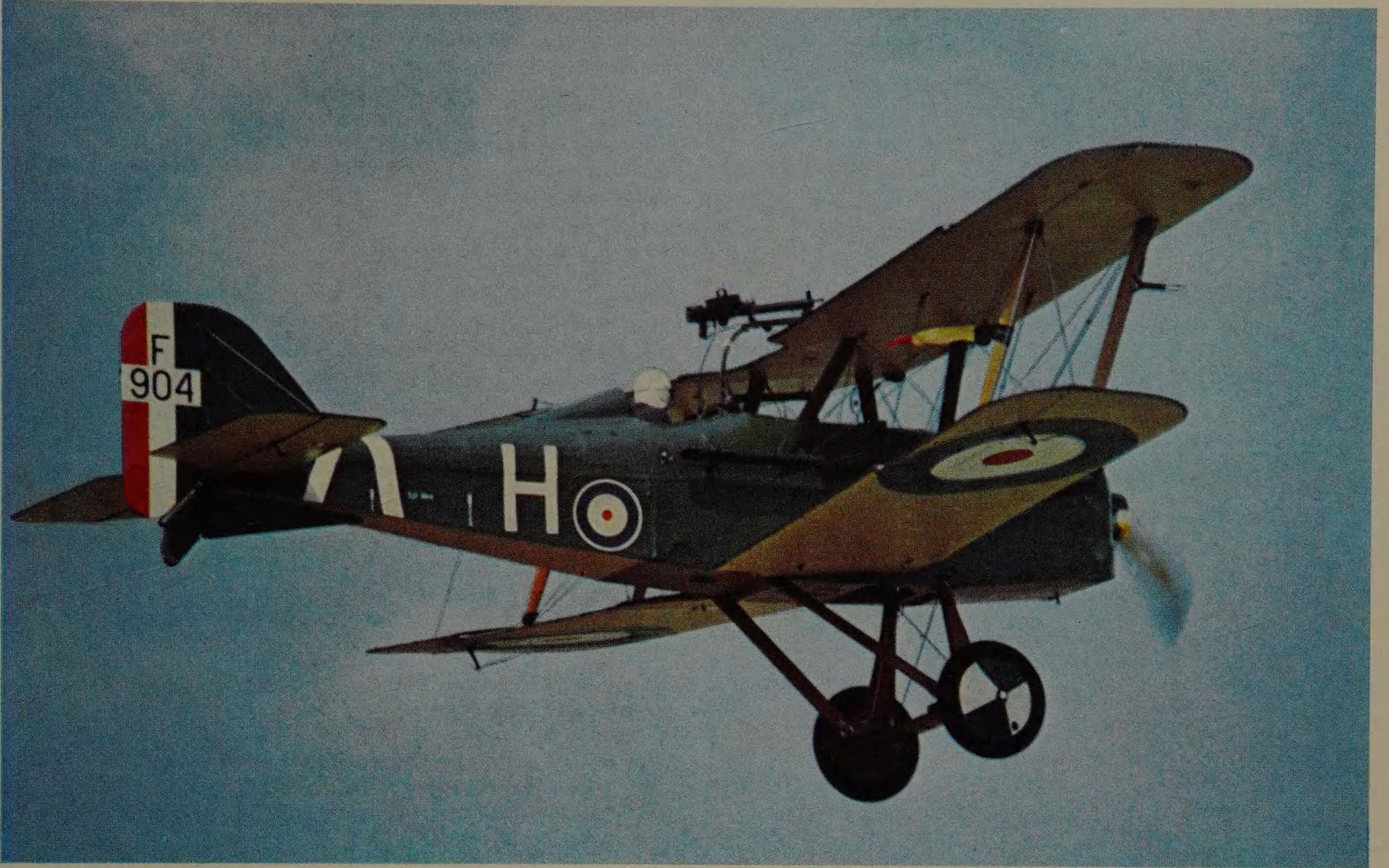
Successful killer: A First World War SE 5a, sometimes claimed to be the outstanding British fighter plane of the 1914-18 war. It had a range of 250 miles, a top speed of nearly 140 mph and twin machine-guns. This one belongs to the Shuttleworth Collection of historic aircraft in England.
