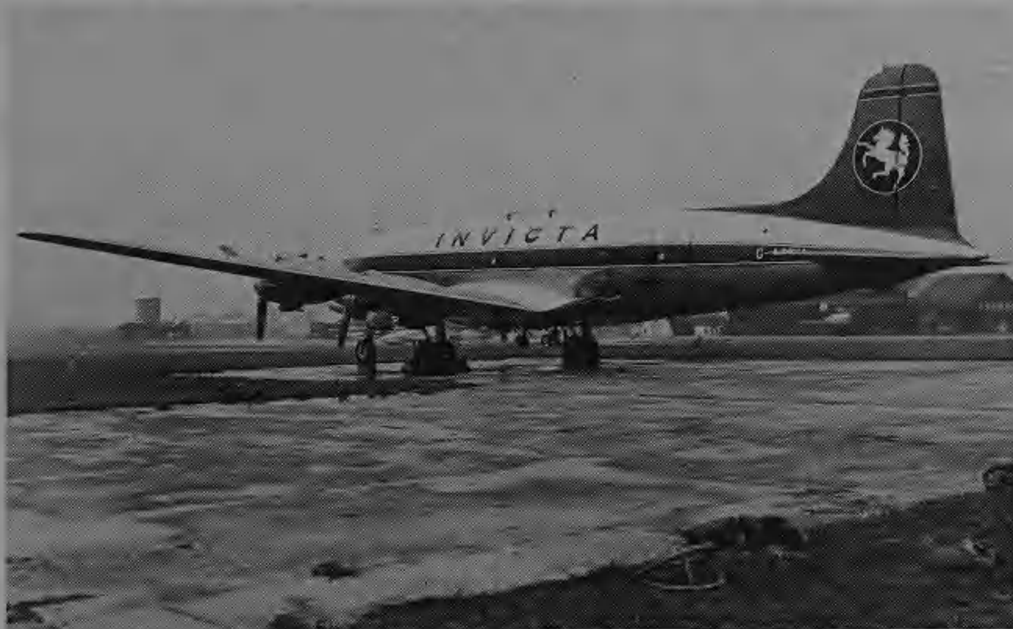
Above: Commercial airliners changed very little in the 25 years after the DC-3 was introduced. They were simply stretched to carry more passengers and given tricycle landing gear. Typical of them was the DC-4 Skymaster which gave its name to the DC-4 Generation of transports.
