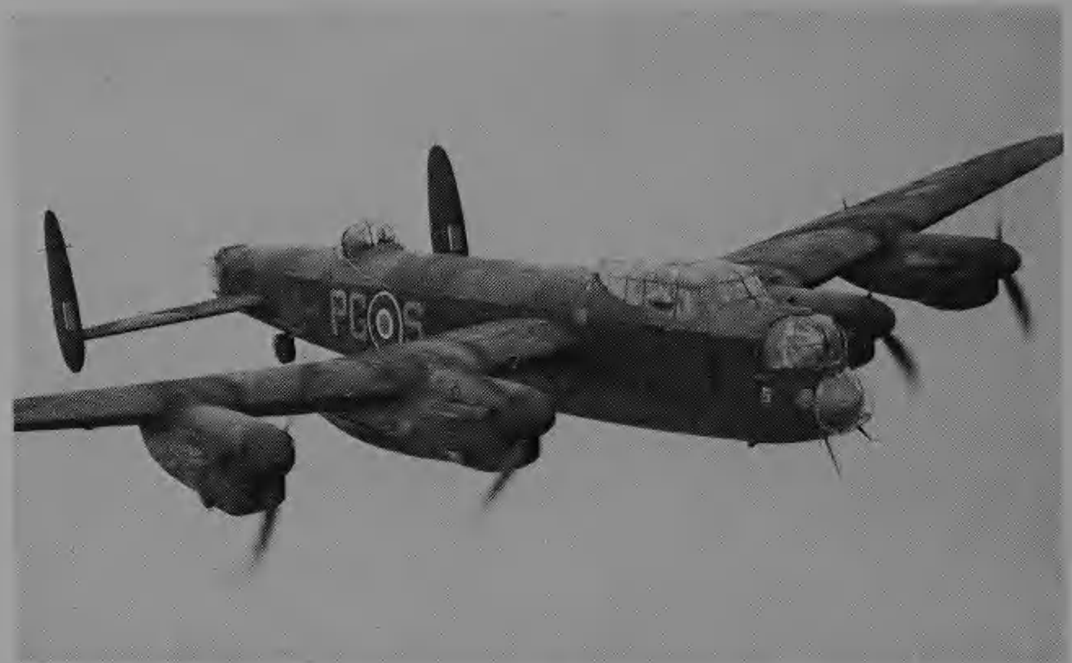
Above: The means of victory, the bomber. The Avro Lancaster is believed by some to have been the most successful heavy bomber of the war. Like the Spitfire, it was also born out of failure. When the twin-engined Manchester bomber was hit by troubles it was decided to alter the design and fit four engines. It resulted in the finest British bomber of the Second World War and one of the most successful aircraft ever built. Between 1942 and the end of the war Lancasters dropped over 608,000 tons of bombs and took part in the epic Dambusters’ raid in May 1943 when aircraft of 617 Squadron breached vital German dams with specially designed bombs. The Lancaster had a 101 ft wing-span, four 1,460 hp engines, a top speed of 287 mph, could carry 22,000 lb of bombs and was armed with ten guns.
