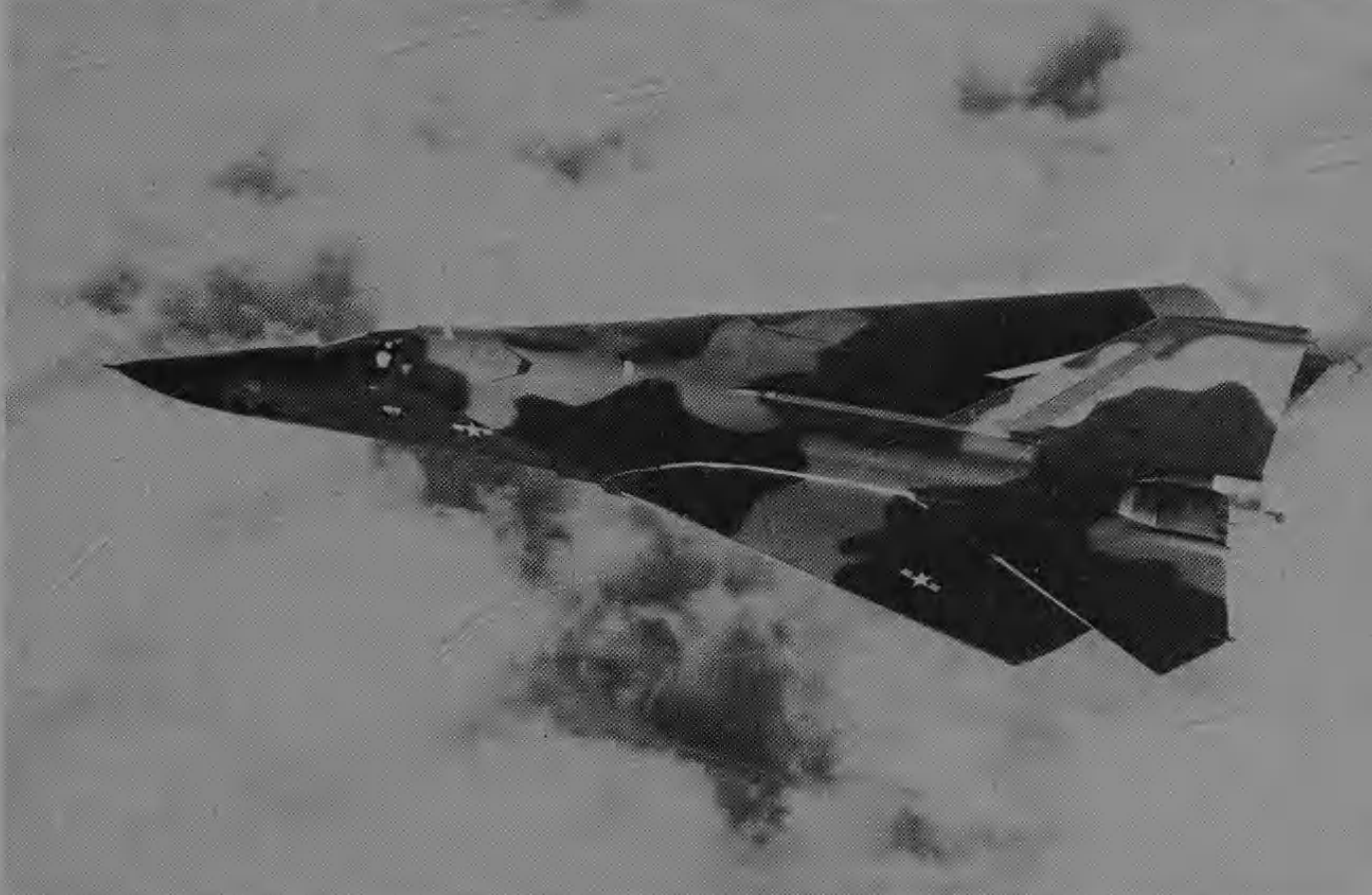
. . . for high-speed flight the wings swing right back to form a delta shape.
