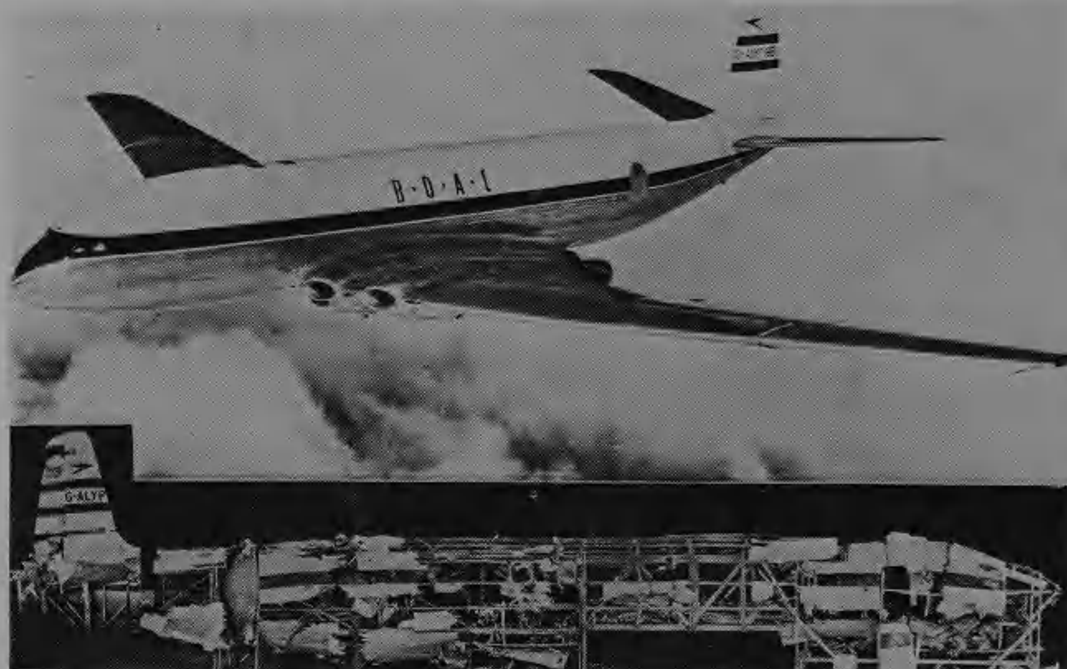
Top: The "perfect lady" which turned out to be wicked: the prototype De Havilland Comet, the world's first jet-powered airliner. Note how square-cut the fuselage windows are.
