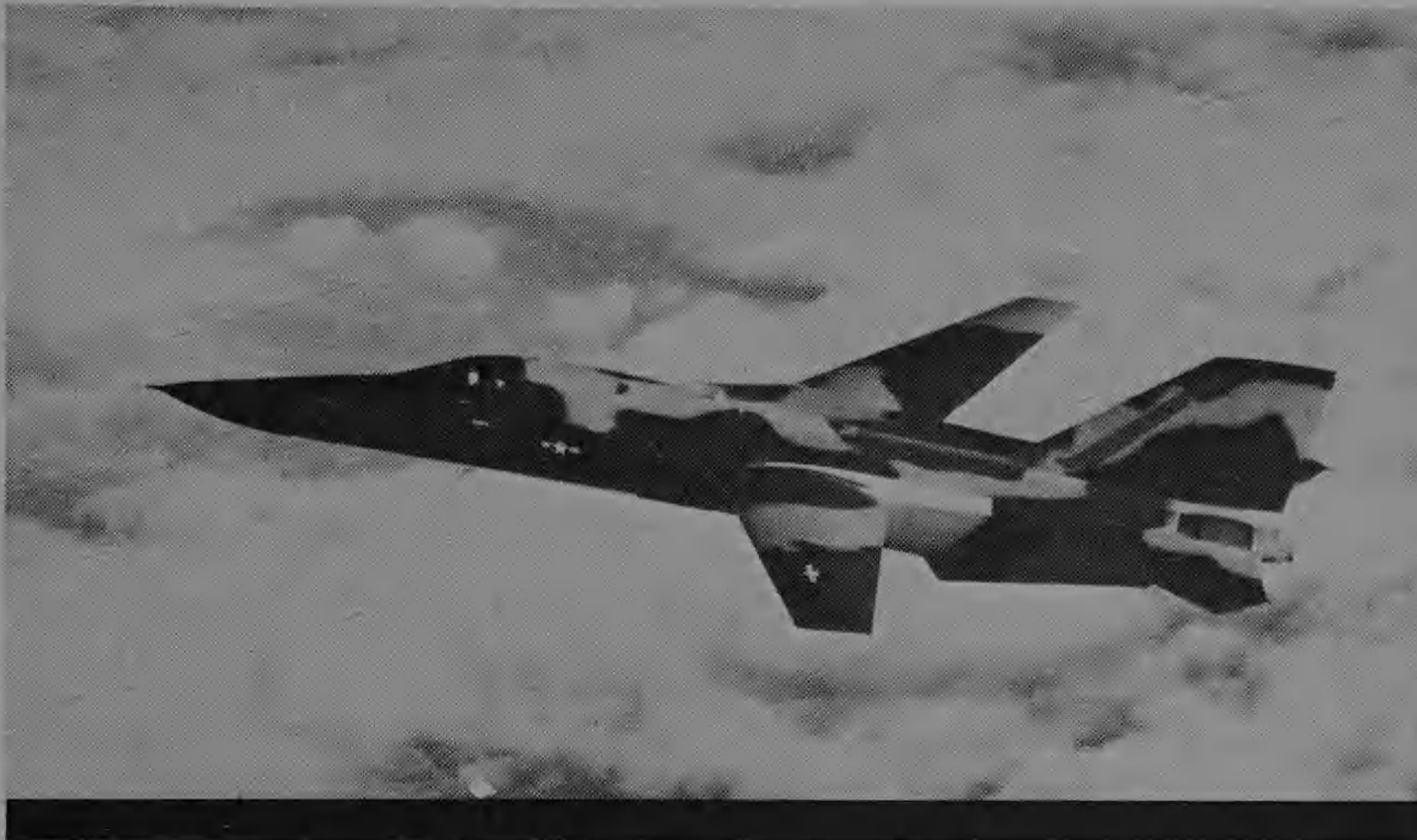
Left: The fastest gun in the West, the F-111. It is the only swing-wing design to have seen active service. For low-speed flight, take-off and landing its wings swing right forward . . .
