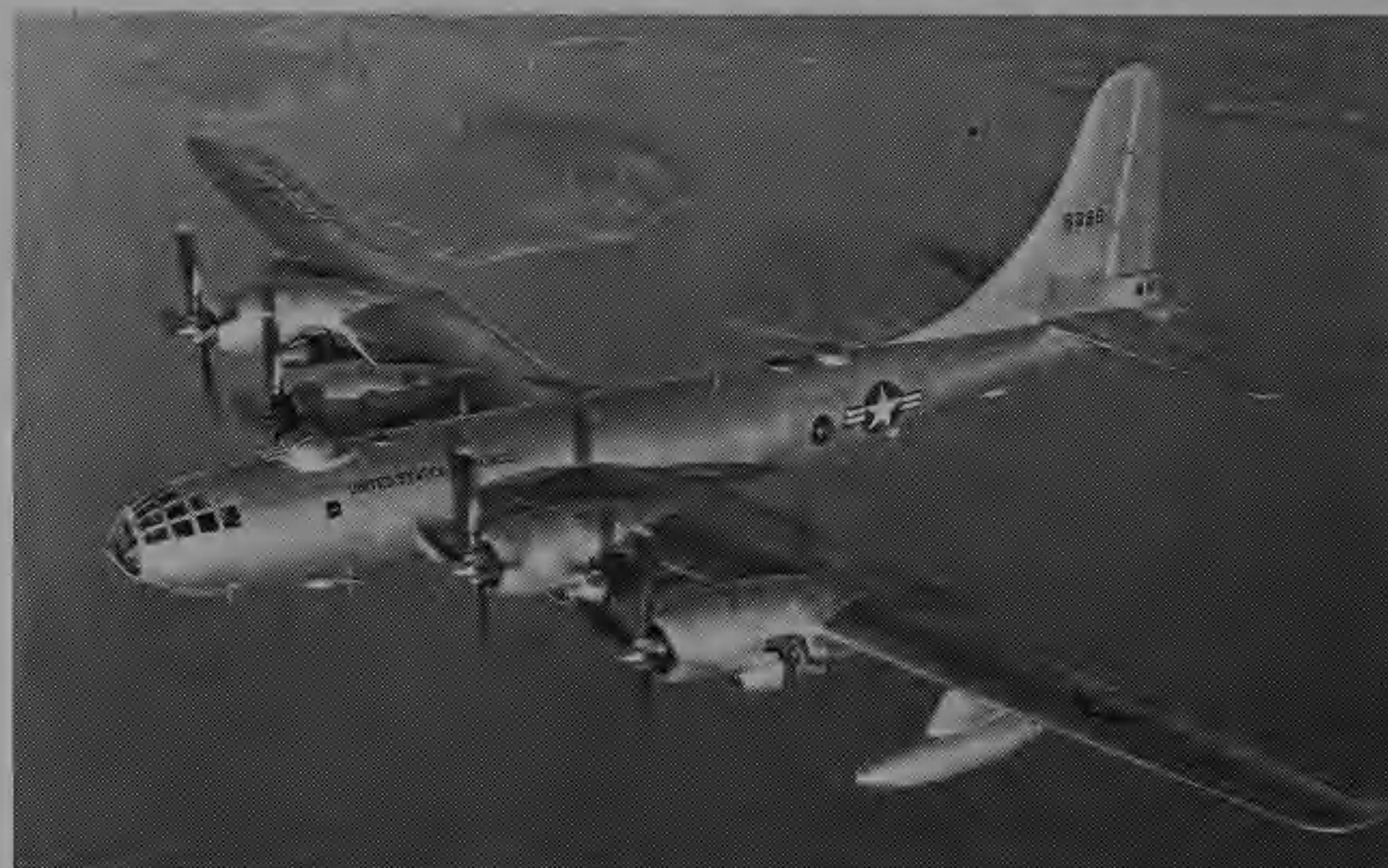
Above: The Boeing B-50, a developed version of the Second World War B-29 Superfortress. One of these aircraft, the Lucky Lady , made the first non-stop flight round the world in 1949.
