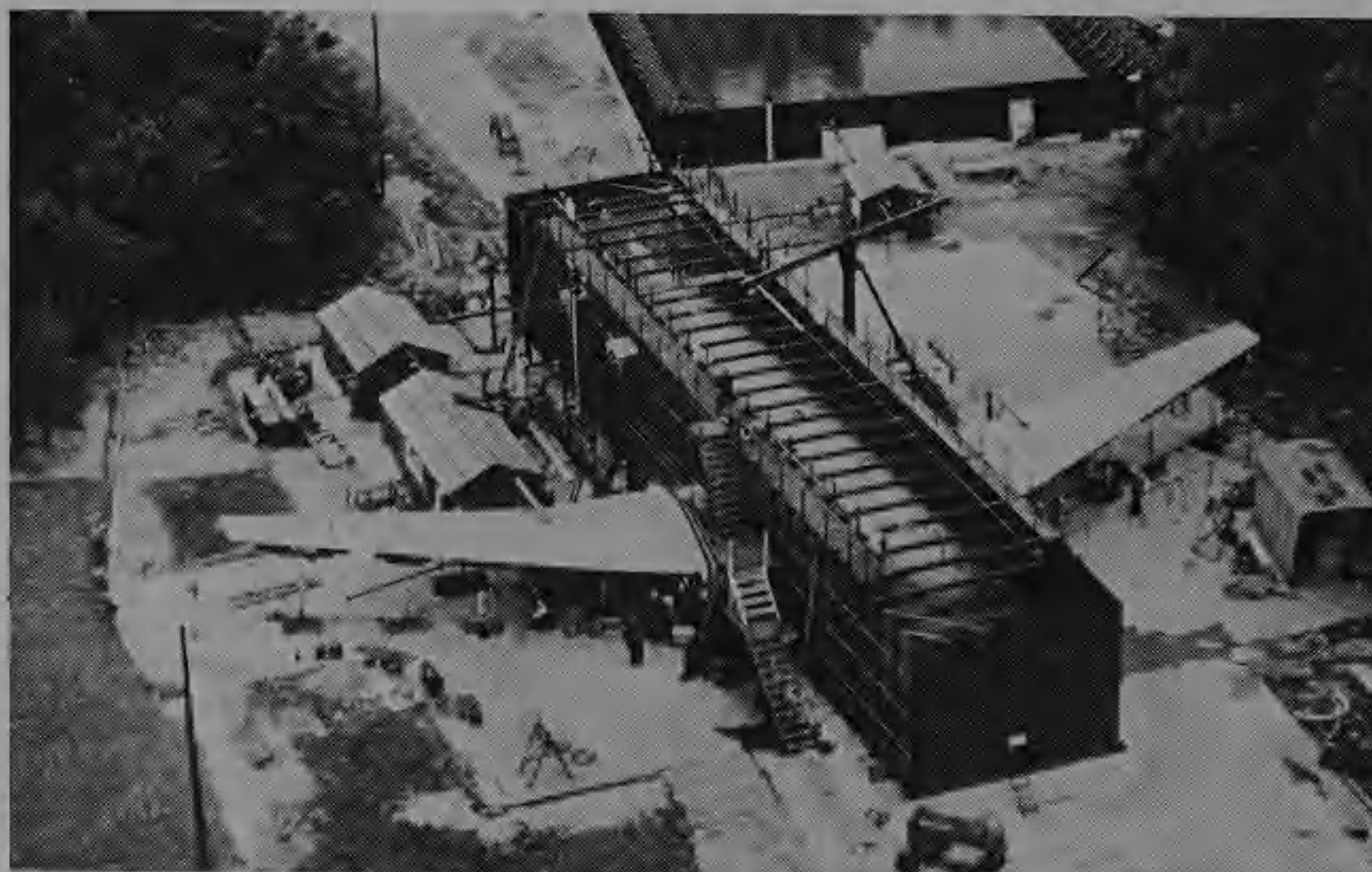
Right: Where they found the answer to the Comet riddle: the fuselage of the test aircraft submerged in the 250,000 gallon water tank where it split after "flying" for 9,000 hours.
