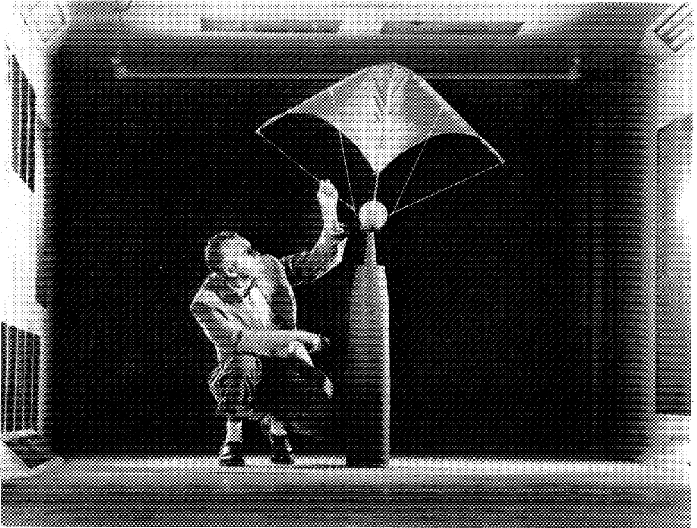
Francis Rogallo of the Langley Research Center adjusts a model of his paraglider, often called a "Rogallo wing," in the 480-kilometer-per-hour wind tunnel. In this 1959 test, the paraglider was being considered as a device to recover stages of the Saturn booster following launch.
