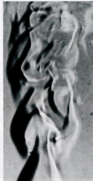
Schlieren photography produces images of density variations in a column of gas.
