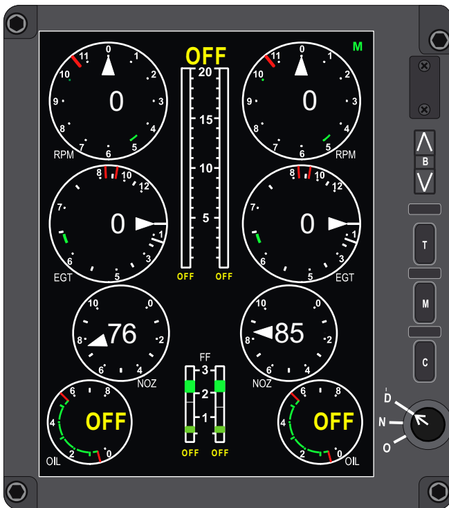
EED NORMAL DISPLAY (BATTERY POWER)
