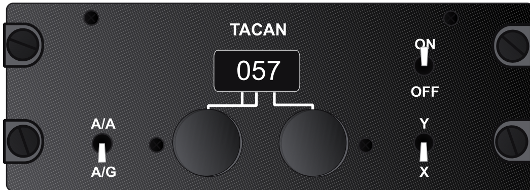
TACAN BACKUP CONTROL PANEL (TCN CHANNEL SELECTED)
