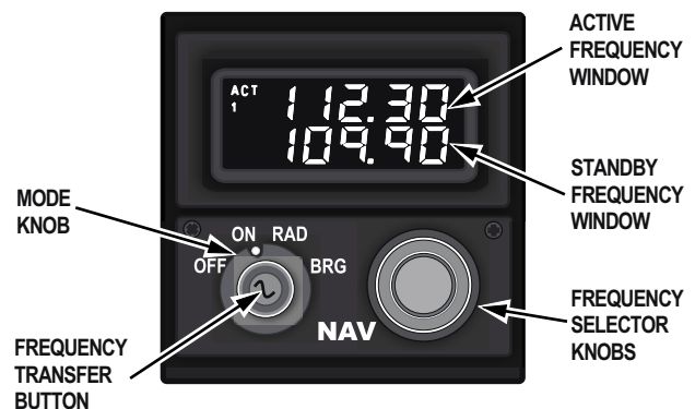
Figure 1-253. NAV Backup Control Panel
