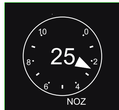
Figure 1-10. Normal Nozzle Position Indicator Oil Pressure (OIL)
