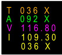
Figure 1-226. MFD NAV Data Block
