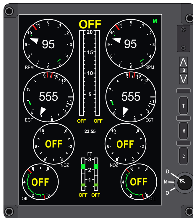
EED NO SOURCE DATA DETECTED FROM EXTERNAL SENSOR (LEFT AND RIGHT NOZ, LEFT AND RIGHT OIL, LEFT AND RIGHT FF, LEFT AND RIGHT FUEL QUANTITY)
