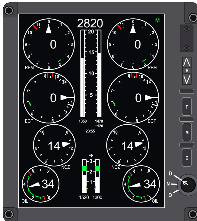
EED NO SOURCE DATA DETECTED FROM EXTERNAL SENSOR (LEFT AND RIGHT RPM, LEFT AND RIGHT EGT)
