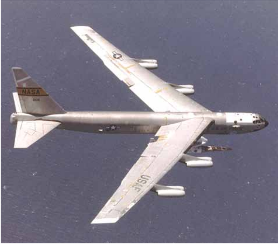
Figure 22: The Boeing NB-52B Stratofortress "008" at DFRC and the first X-43A Hyper-X scramjet test bed on a "captive carry" test flight over the Pacific Ocean, April 2001. NASA Image EC01-0126-07
