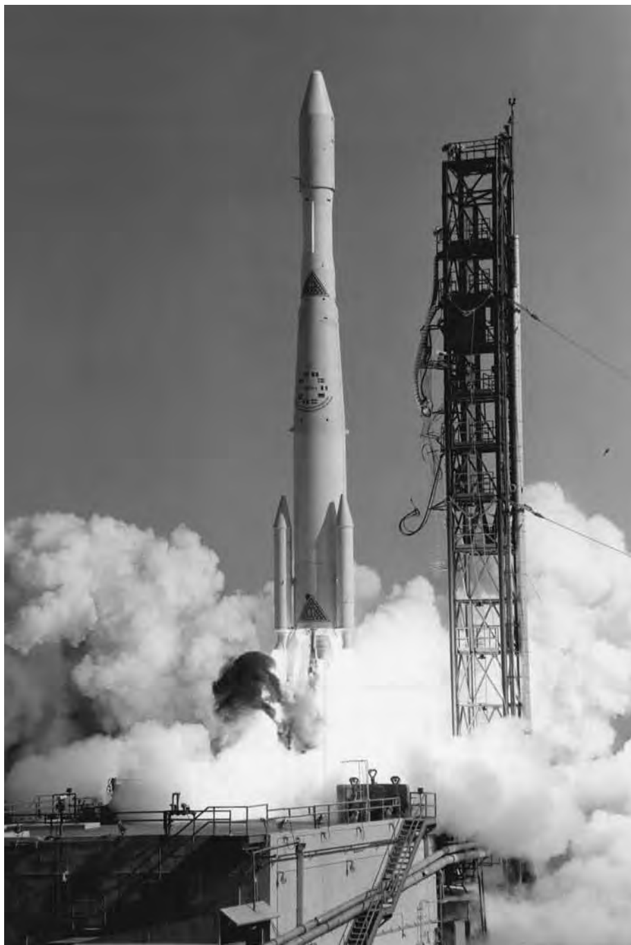
Figure 1: A Delta E rocket launching from KSC on 5 December 1968 carrying Highly Eccentric Orbit Satellite 1 for the European Space Research Organization. Notice the strap-on motors at the base of the Delta. NASA
