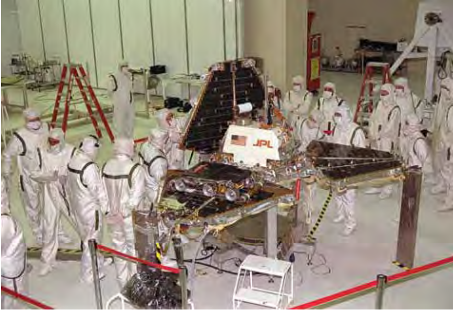
Figure 1: Strong in-house technical capability formed the basis for NASA's original organization culture. Here, Jet Propulsion Laboratory employees close the metal petals of the Pathfinder lander dispatched to Mars in 1996. The Sojourner small rover is visible on one of the three petals. NASA Image 96PC-1130
