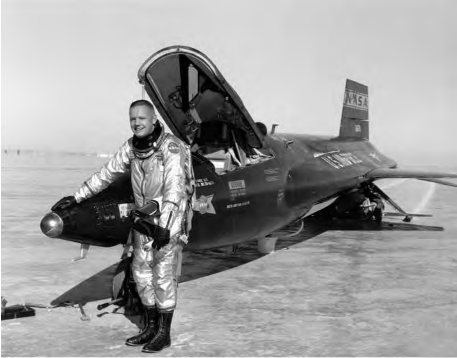
Figure 9: Dryden pilot Neil Armstrong is seen here next to the X-15 after a research flight. The X-15 was a rocket-powered aircraft 50 feet long with a wingspan of 22 feet, flown over a period of nearly 10 years, from June 1959 to October 1968. On 22 August 1963, Joe Walker flew the X-15 to 354,200 feet (67 miles or 107 kilometers) to set the world altitude record for winged vehicles. Research from the X-15 project was vital to the design and construction of the Space Shuttle and also contributed to the development of the Mercury, Gemini, and Apollo piloted spaceflight programs. The X-15s made a total of 199 flights. NASA Image E60-6286
