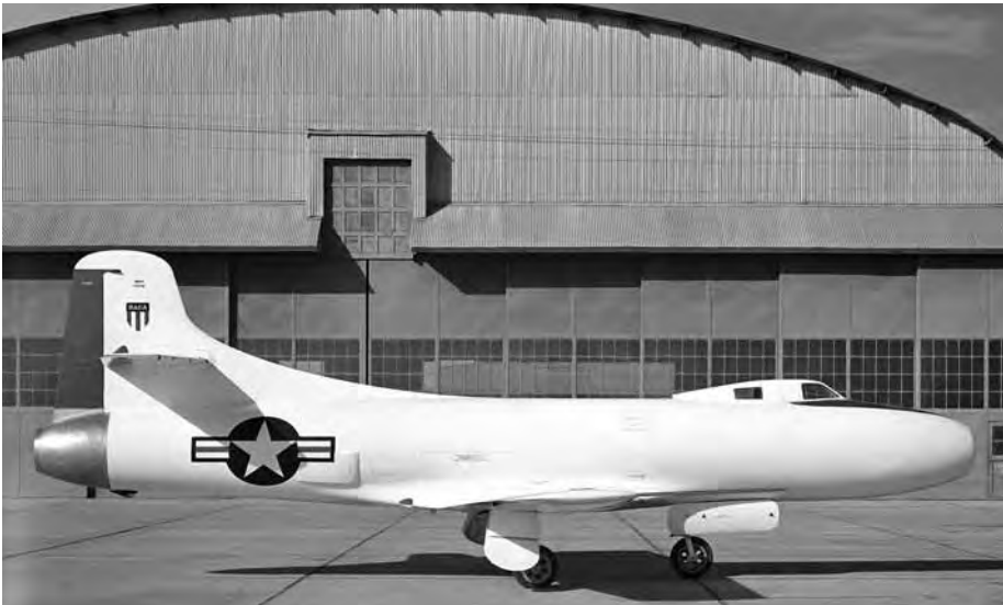
Figure 5: The Navy-sponsored, turbojet-powered Douglas D-558-1 Skystreak. This is the third D-558-1 (USN 37972); its slender lines earned it the nickname "The Flying Test-tube." NASA Image E49-090
