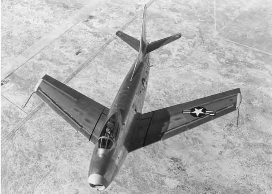
Figure 9: The North American Aviation XP-86 Sabre, the first jet-propelled airplane to exceed Mach 1 (in a dive), 1948. Air Force Flight Test Center History Office
