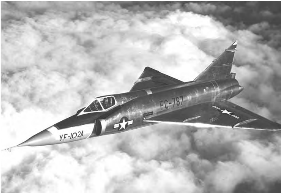
Figure 14: The YF-102A, with area ruling, longer length (hence higher fineness ratio), and shock bodies flanking the tail cone. AFFTC
