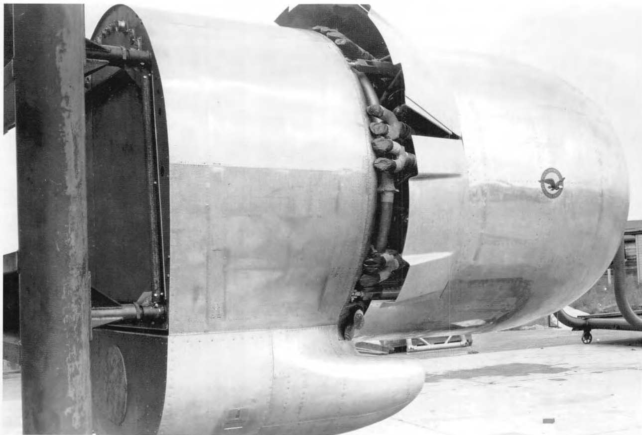
An interesting feature of this photograph is the divided tailpipe for each exhaust stack. (Courtesy of Pratt & Whitney)
