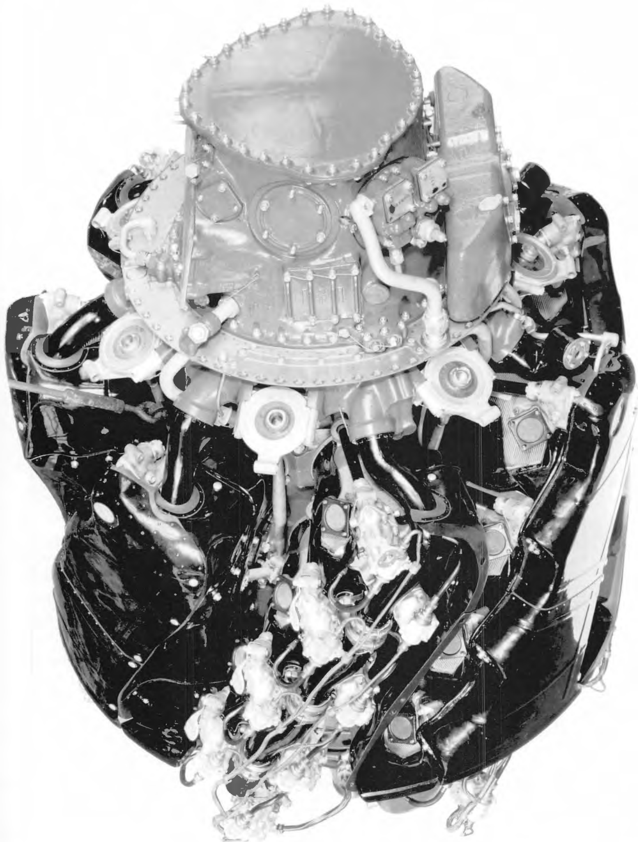
R-4360-65. A view from the other side reveals another hooded baffle removed; this time the front and rear halves.
