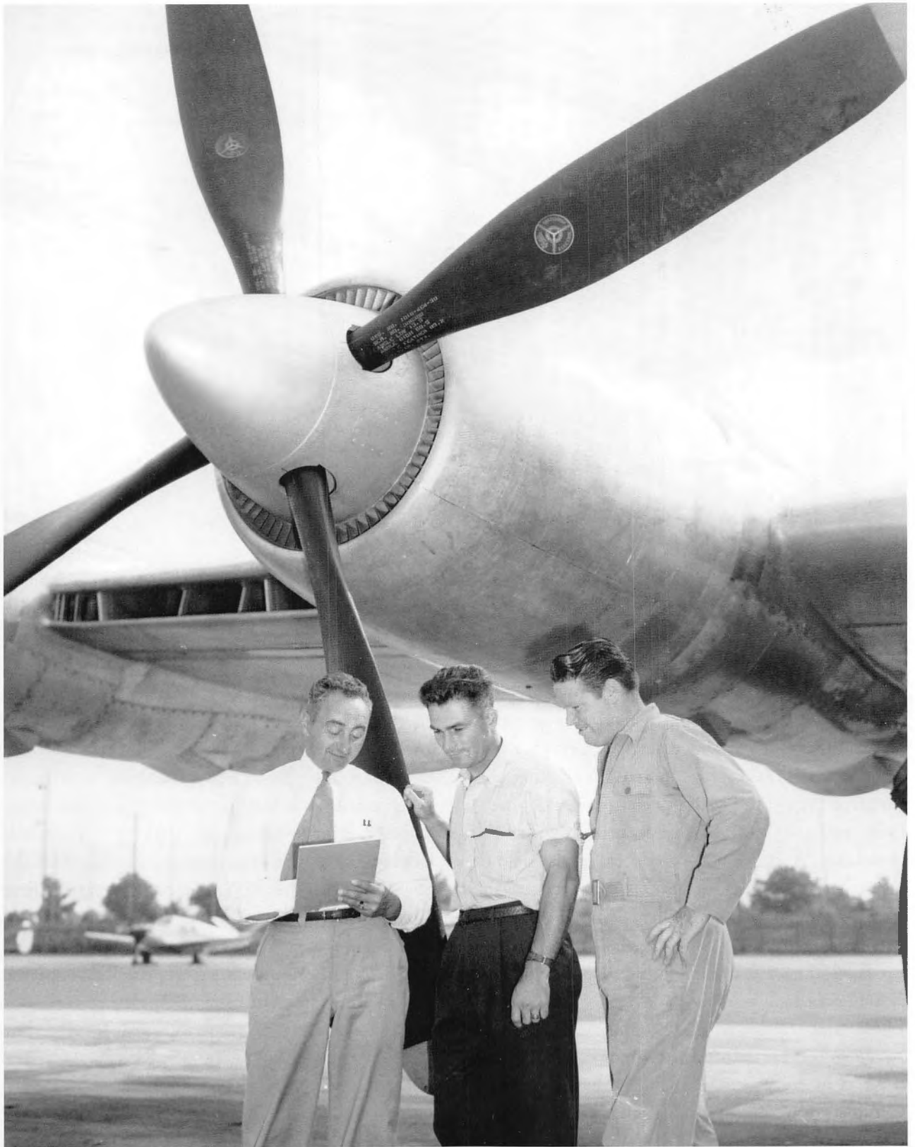
One of the nicest R-4360 installations was the one used for the Republic XF-12 Rainbow. Of interest in this shot is the good view of the engine cooling fan and leading-edge intakes for the oil cooler, intercooler, and induction. (Courtesy of Warren Bodie)
