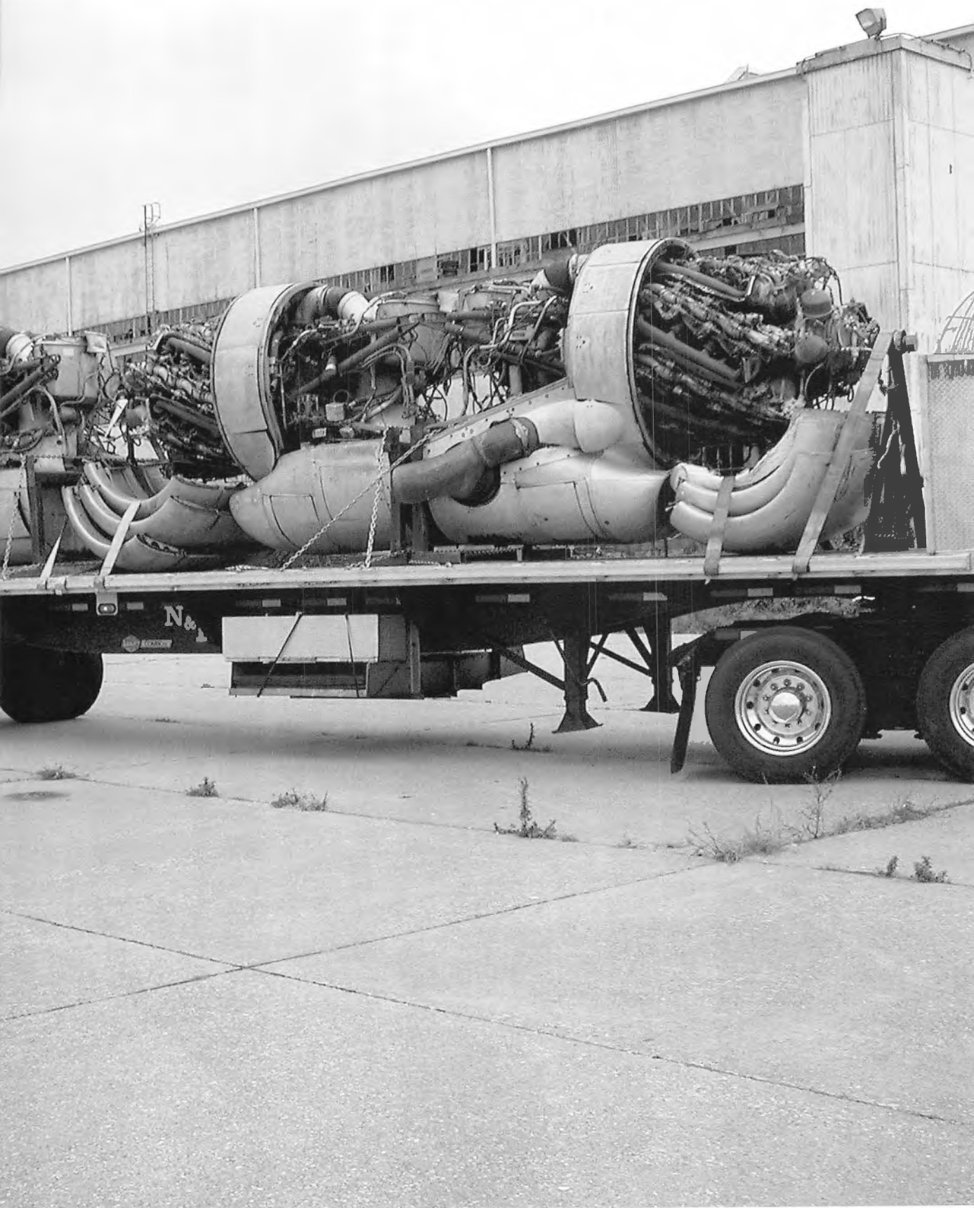
Six QECs were rescued from C-97G 53-3816 just prior to its scrapping. This photo shows one of the two tractor-trailer loads. (Courtesy of Tim Chopp, Berlin Airlift Historical Foundation)
