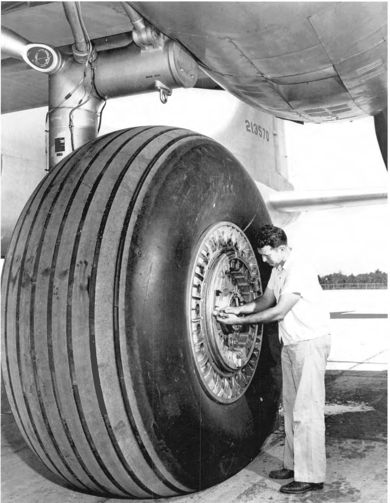
Little wonder that only a handful of runways around the world could handle the enormous weight of the XB-36, particularly when the majority of that load was only distributed on two tires. (Courtesy of National Archives & Records Administration)
