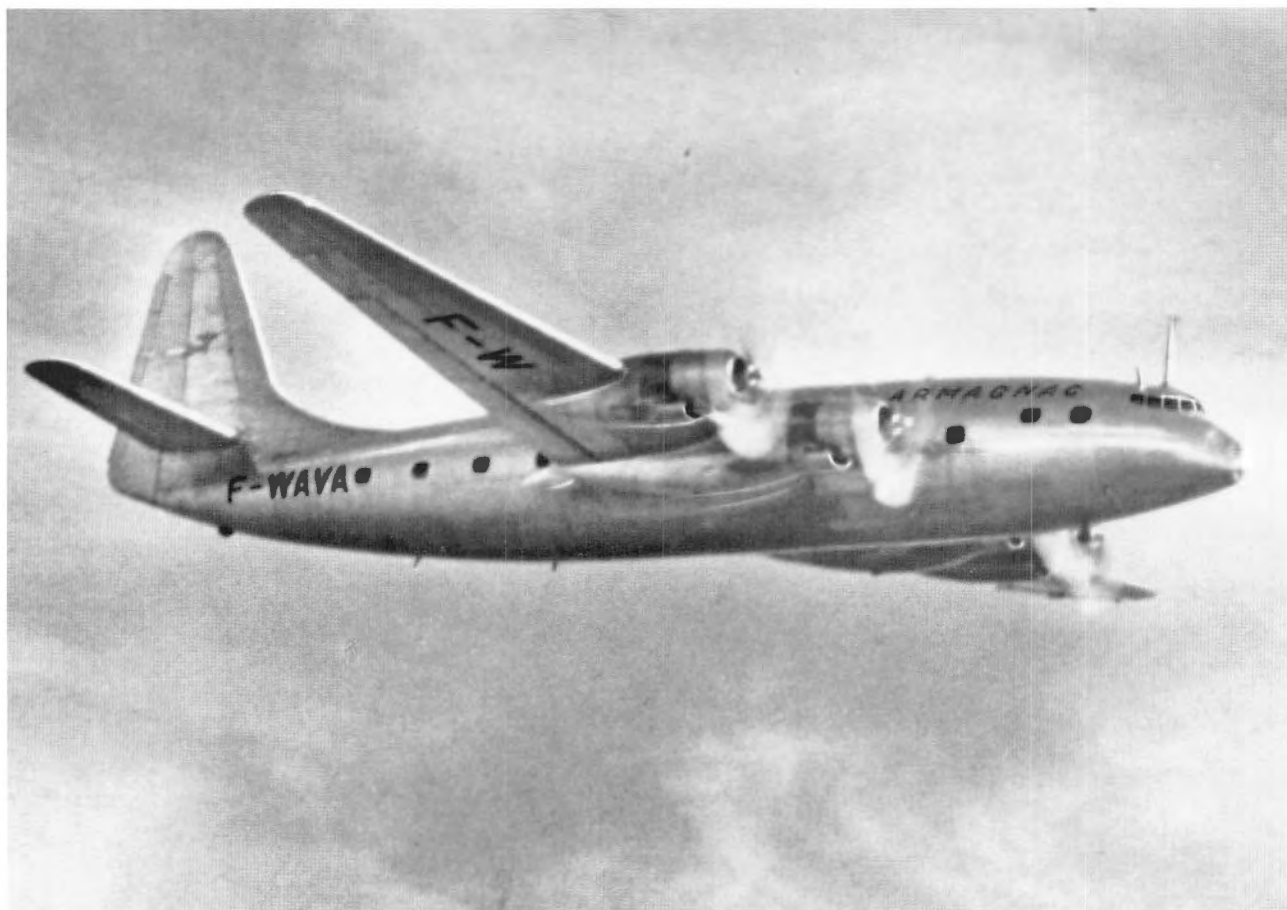
Aero-Sud-Est SE-2010 in flight. This grainy, poor quality photo illustrates the conventional lines of this unsuccessful commercial aircraft. Seems like a waste of four good R-4360s. (Courtesy of Pratt & Whitney)
