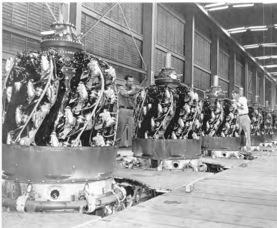
Left: B-36 engines being inspected prior to crating for shipment to the customer—the U.S. Air Force. (United Technologies Corp./Pratt & Whitney)
