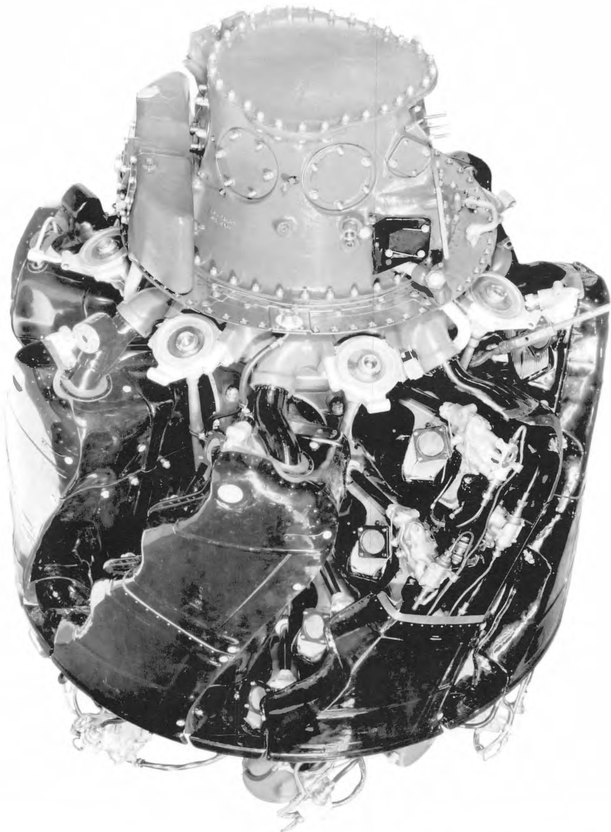
R-4360-65. It would appear that Pratt & Whitney used the same engine for this series of portraits for the R-4360-65. Note the same rear half hooded baffle is missing as that in the image on top of page 285.
