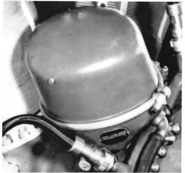
Photograph of one of the four magnetos that make up a low-tension ignition system. This was a much simpler, albeit still complex, system. Its high-altitude capability was a savior for aircraft such as the B-36. Unlike low-tension schemes used on other engines, the R-4360's system employed a boost coil for each spark plug. ( United Technologies Corp./Pratt & Whitney )
