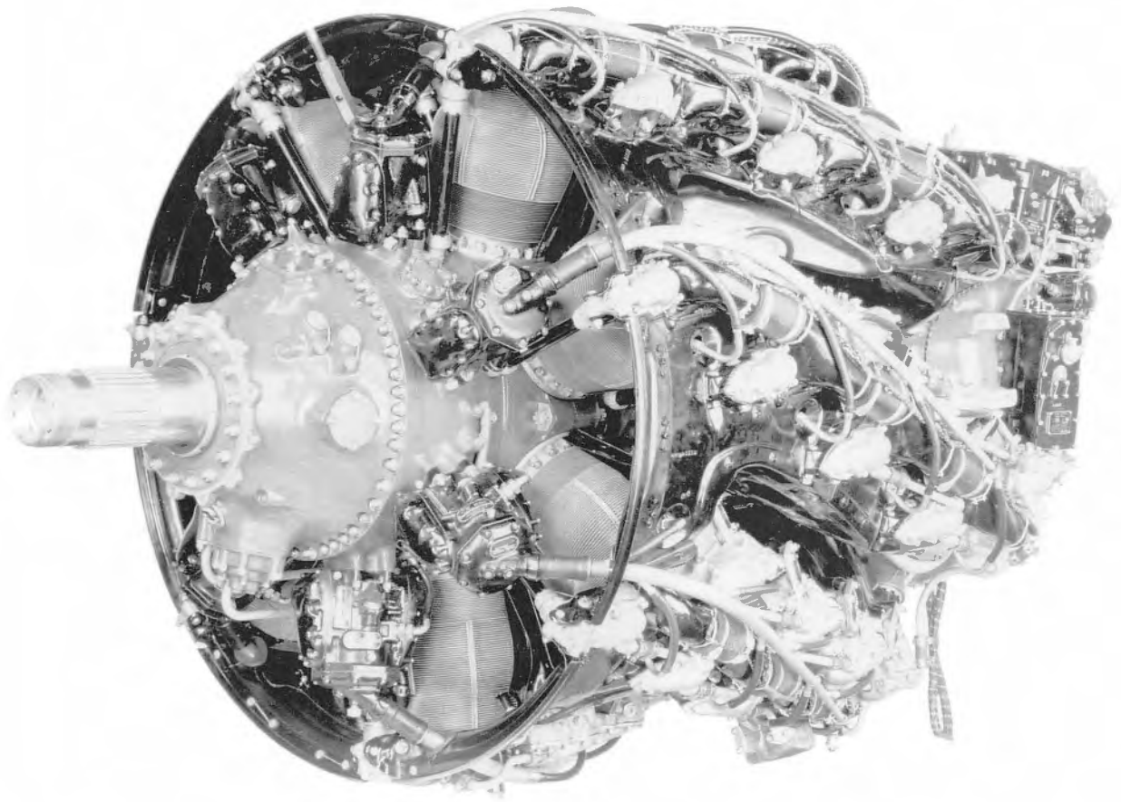
This R-4360-27 was the production version of the R-4360-15. -27s were used to power Douglas C-74 transports. ( United Technologies Corp./Pratt & Whitney )
