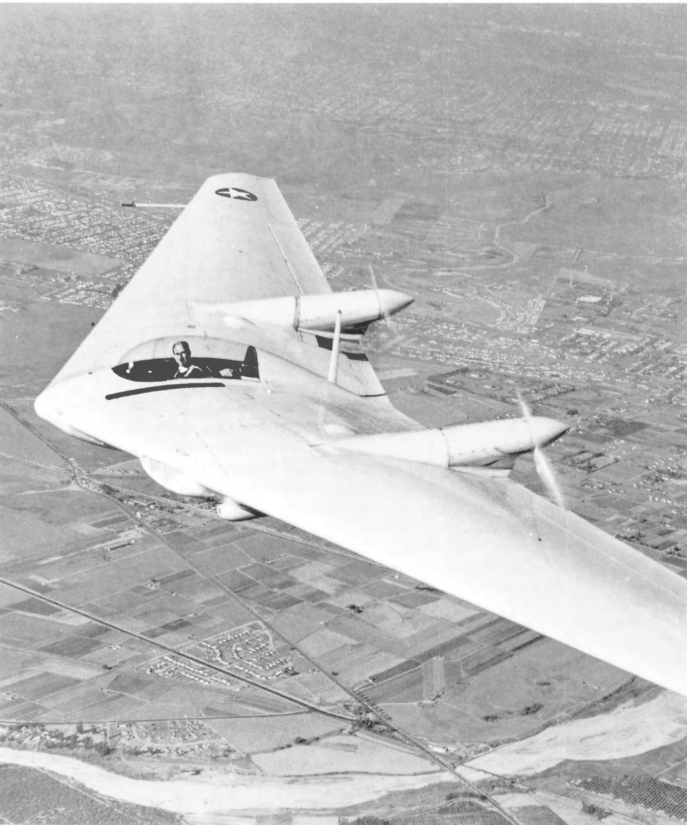
For XB-35 development, Jack Northrop had four \frac{1}{8} -scale proof-of-concept flying wings built designated N-9M. (Courtesy of National Archives & Records Administration)
