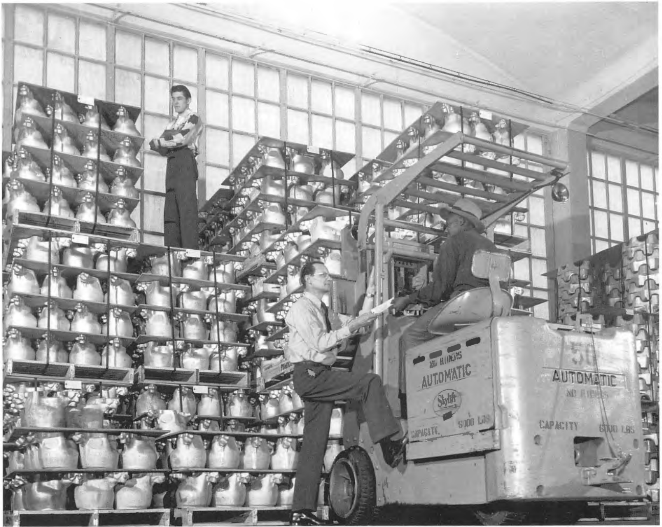
Pallet loads of cylinder head forgings ready to have their cooling fins machined in. This particular photograph was taken at Ford Motor Company's facility. Note the crankcase sections in the background also ready for machining operations. (From the Collections of Henry Ford Museum & Greenfield Village)
