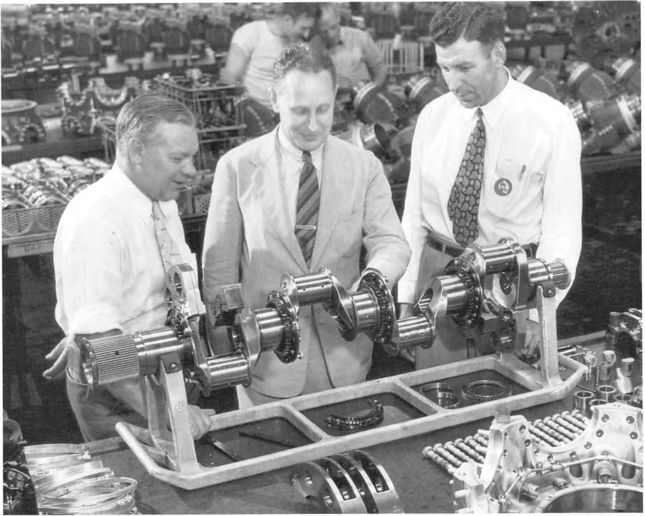
This is a photograph taken in Pratt & Whitney's East Hartford facility. The crankshaft is the heart of the engine and this is where final assembly begins. (United Technologies Corp./Pratt & Whitney)
