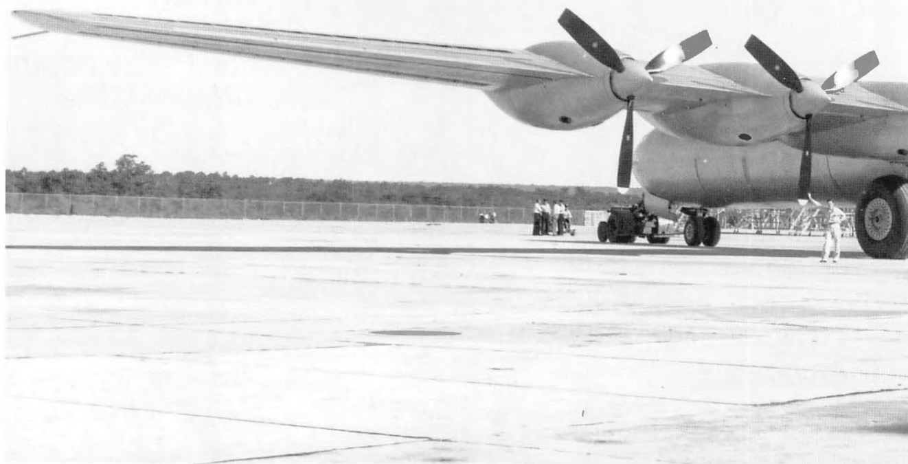
Convair's XB-36 sitting on the ramp. Note the huge single-wheel main gear—soon replaced by a four-wheel bogie design. (Courtesy of National Archives & Records Administration)
