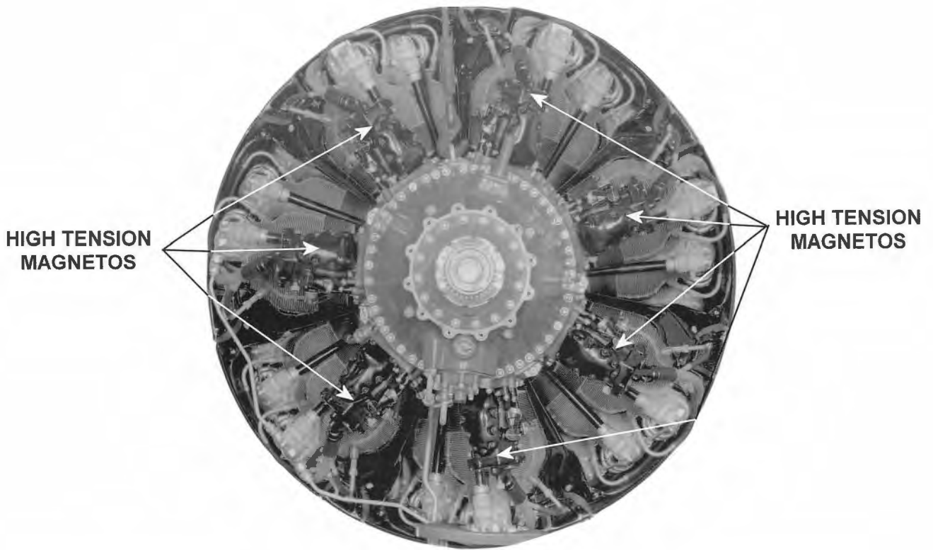
This is how the front of the engine appears when fitted with a high-tension ignition system. ( United Technologies Corp./Pratt & Whitney )
