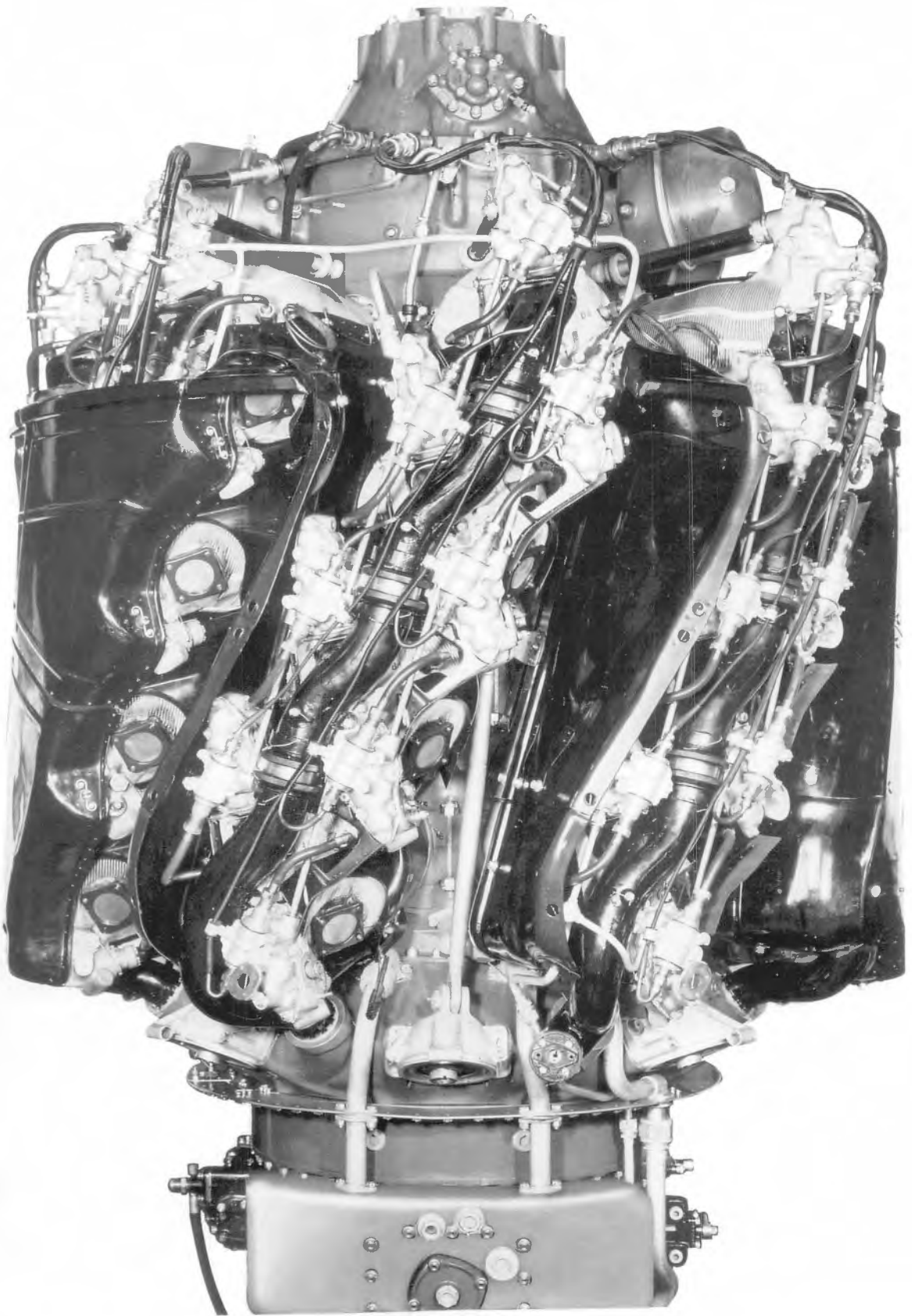
R-4360-63. Another bottom view, however, this one shows two hooded baffles removed exposing the cylinder heads and ignition boost coils.
