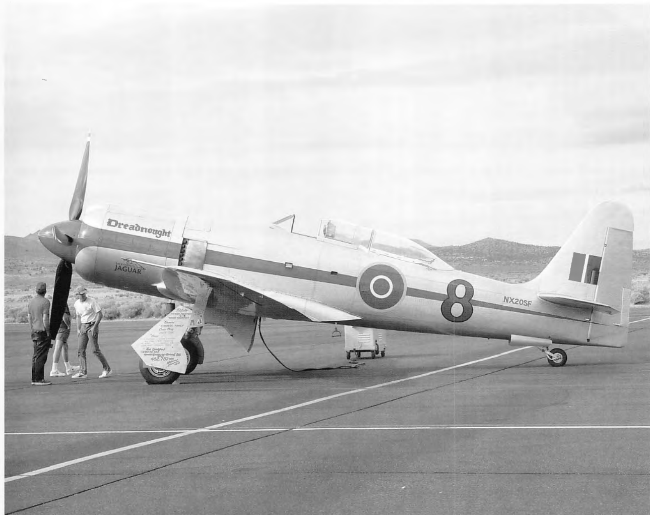
Owned and flown by Dennis and Brian Sanders, Dreadnought , the R-4360-63A-powered Hawker Sea Fury, has appeared at Reno and other racing venues for many years. (Photo by author)
