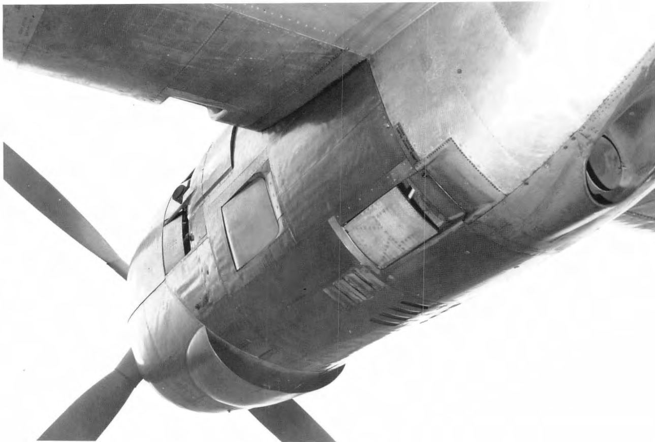
Underside view of a Constitution nacelle. Note the nicely designed exhaust outlet, which offered some degree of jet thrust. (Courtesy of Pratt & Whitney)
