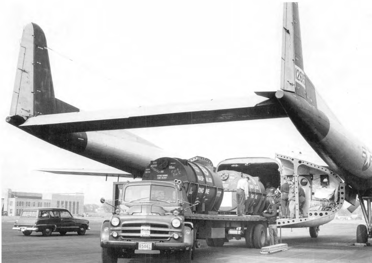
Two R-4360s in shipping cans are being loaded aboard a C-119. The vertically hinged doors could be removed if necessary for flight operations. (Courtesy of National Archives & Records Administration)
