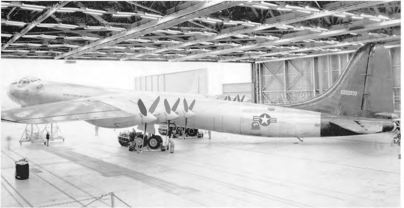
This early production B-36B does not have the J47 jet pods. 120 B-36Bs were later converted to B-36D status, which included the jet pods. (Courtesy of National Archives & Records Administration)
