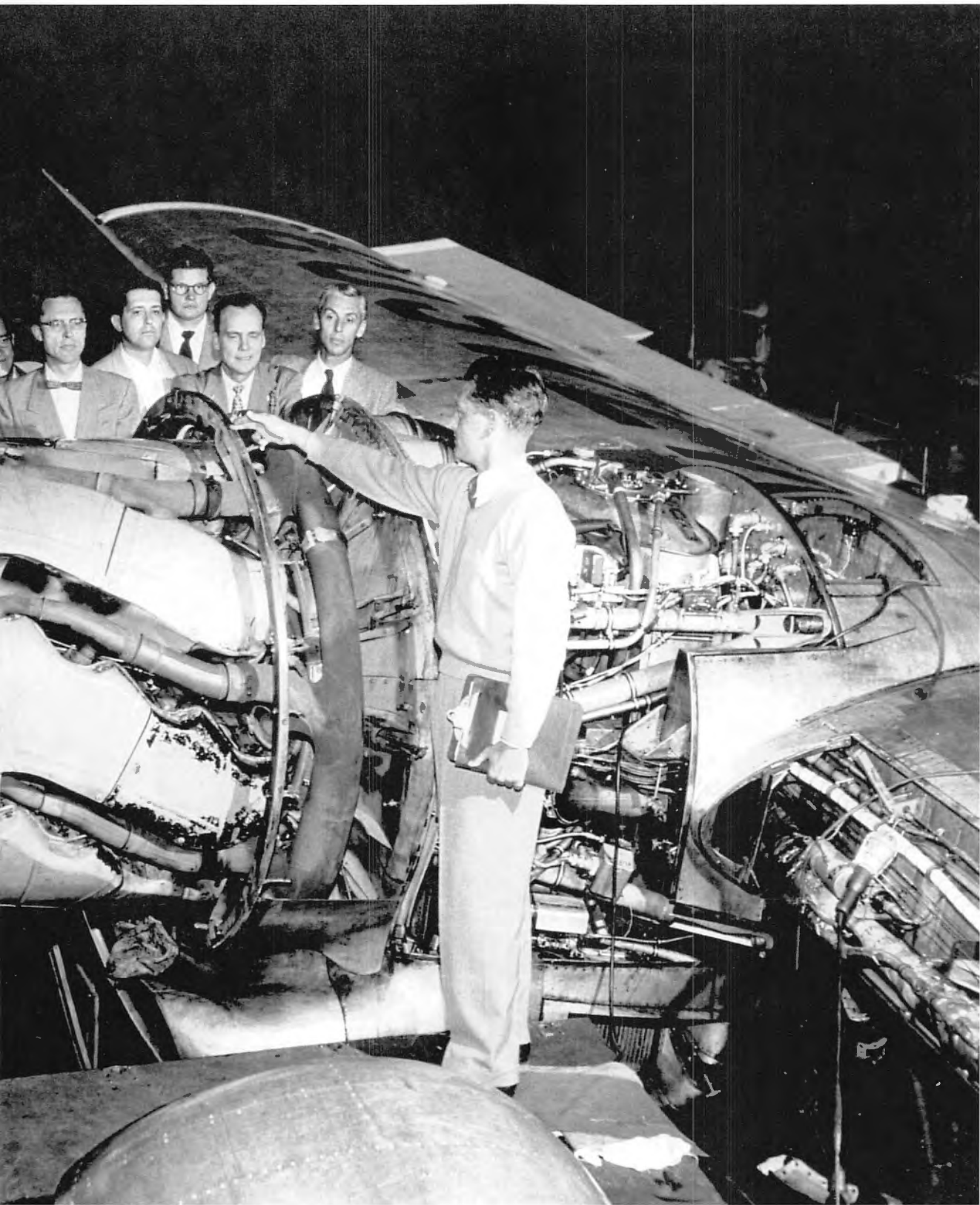
Judging by the suits and ties in this photo, one would have to assume that this may be a sales and marketing pitch. Regardless of why these folks are gathered around the engine, it offers a good idea of how the R-4360 was installed in the B-377. (Courtesy of Pratt & Whitney)
