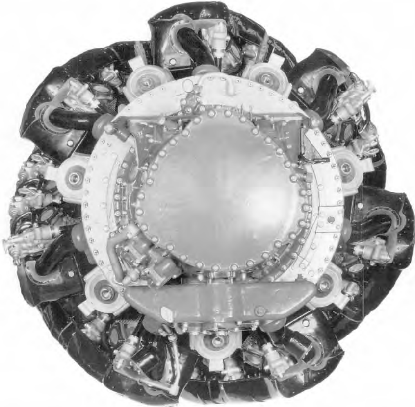
Rear view of the R-4360-65. Note the seven mounts used to support the engine in the airframe. This significant design challenge was a major accomplishment.
