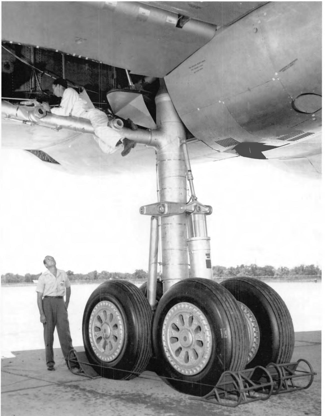
That's more like it! When the B-36's main gear was redesigned into a four-wheel bogie, it opened up far more runways capable of handling its weight. (Courtesy of National Archives & Records Administration)
