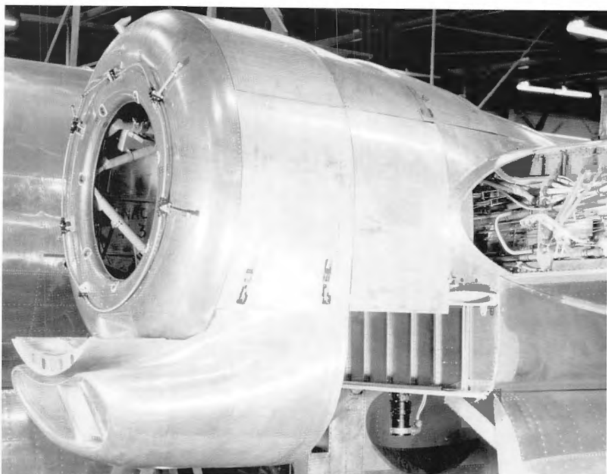
Above: Pratt & Whitney engineers were forced into using the basic nacelle dimensions of the B-29's Wright R-3350. Nevertheless, they pulled off the seemingly impossible by converting a pig's ear into a silk purse. (Courtesy of National Archives & Records Administration)
