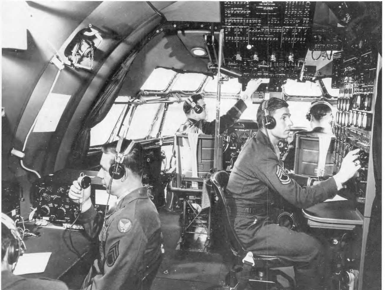
Well laid out flight deck of the C-97 showing the pilot, co-pilot, flight engineer, and radio operator. (Courtesy of National Archives & Records Administration)
