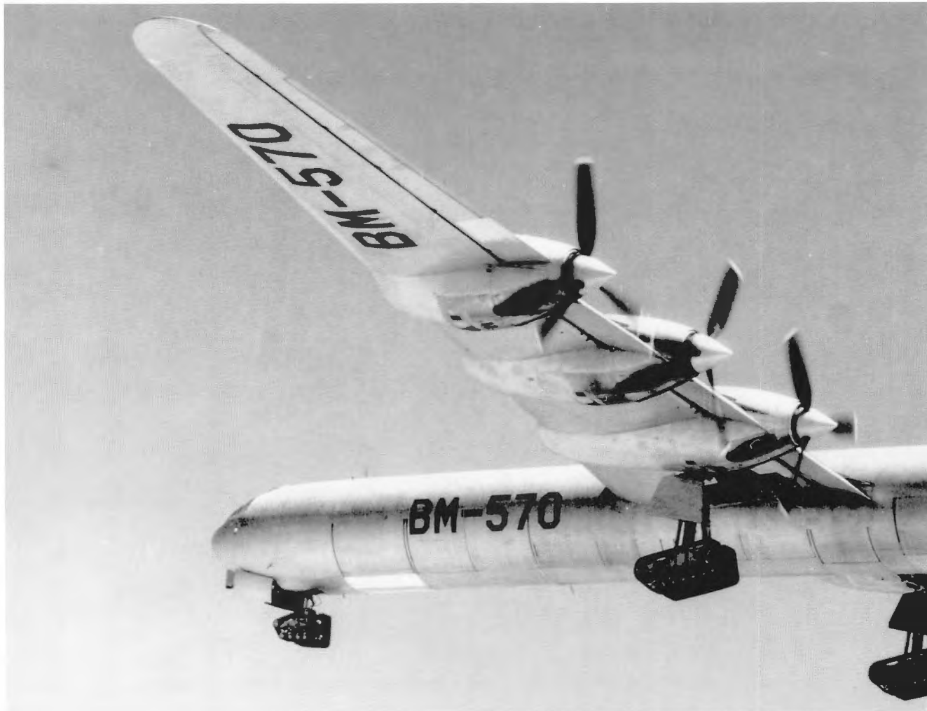
Experiments with main landing gear didn't end with the four-wheel bogie. In an effort to further reduce its bearing loads, a tracked gear was fitted to the XB-36. It flew once. (Courtesy of National Archives & Records Administration)
