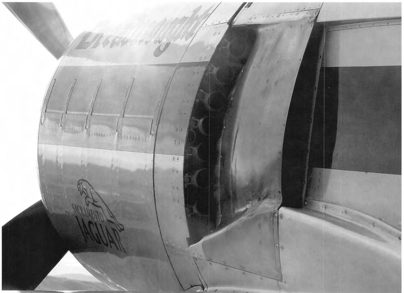
Using exhaust energy to the fullest, Dreadnought uses the classic siamesed jet stack system. Seven outlets on each side of the aircraft are used. (Photo by author)
