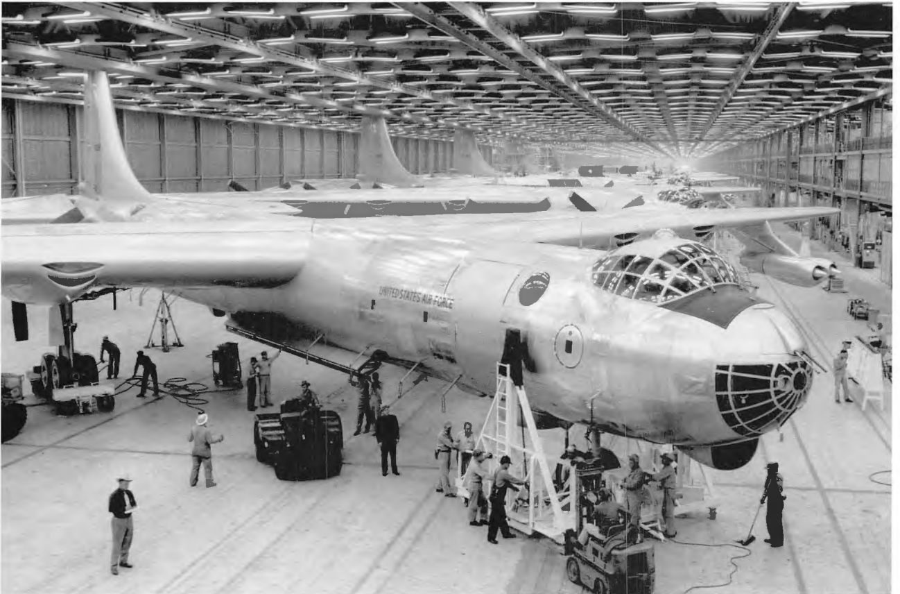
B-36Ds with J47 jet pods rolling down the manufacturing line. (Courtesy of National Archives & Records Administration)
