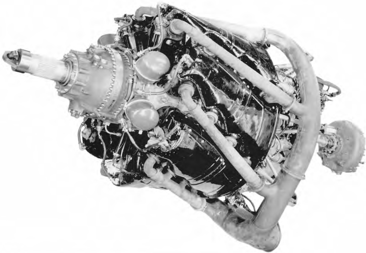
R-4360-57. Intended for the B-36C, this 4,300-hp VDT engine never entered production.
