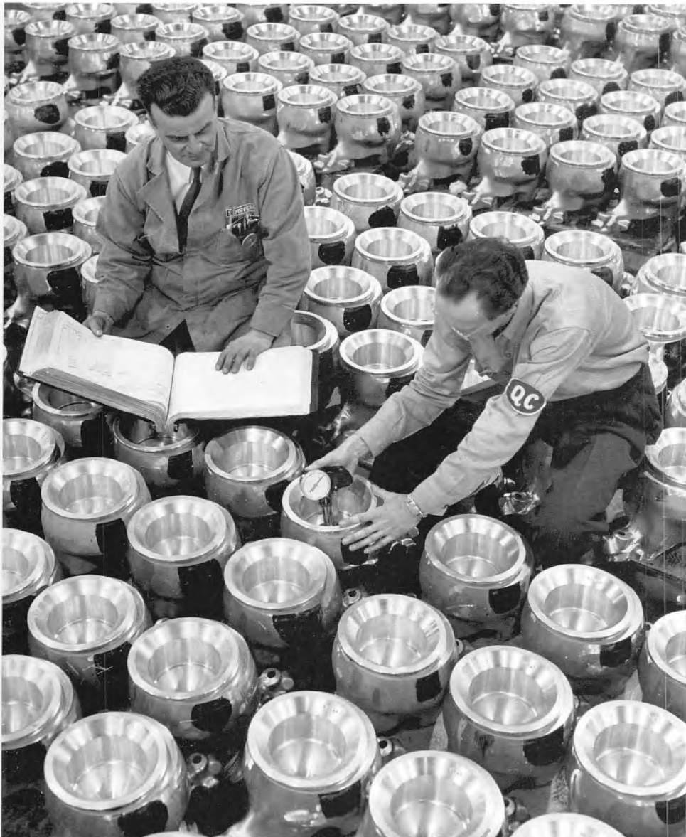
Ford Motor Company personnel inspecting cylinder heads prior to having their cooling fins machined in. It should be noted that with any aircraft engine component, each manufacturing step is inspected. By the time a complex part, such as a cylinder head, is complete it has undergone numerous inspections. ( From the Collections of Henry Ford Museum & Greenfield Village )
