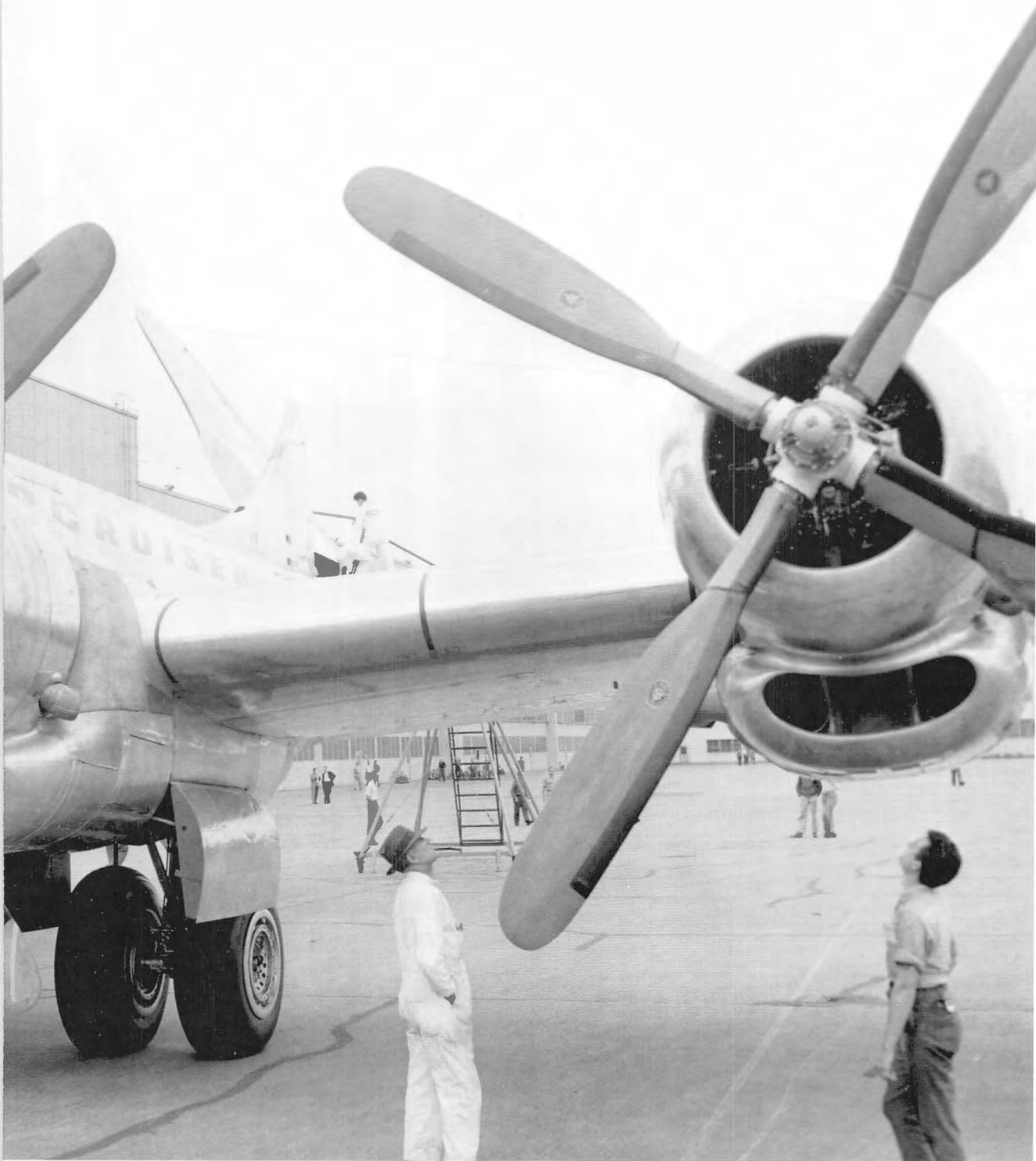
This photo shows the optional Curtiss Electric propellers identifiable by their rounded tips. (Courtesy of Pratt & Whitney)
