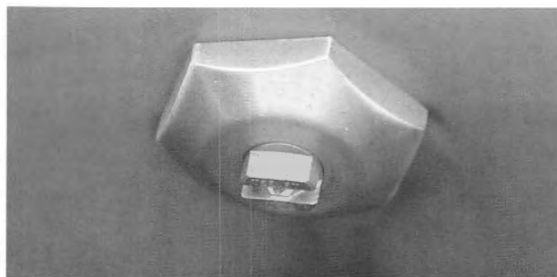
This is a close-up of one of the seven spray nozzles used by Furias to spray water on the cylinders. (Photo by author)
