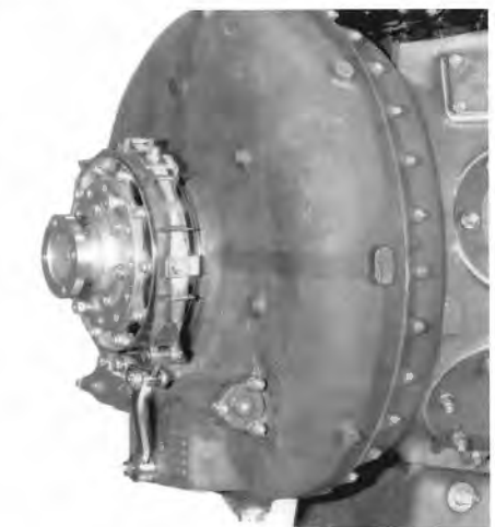
Close-up photo of the fan brake assembly and fluid coupling drive. ( United Technologies Corp./Pratt & Whitney )
