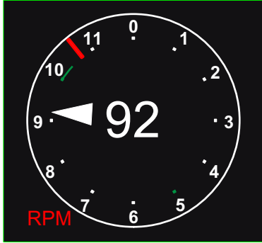
Figure 1-8. Latched RPM Exceedance
