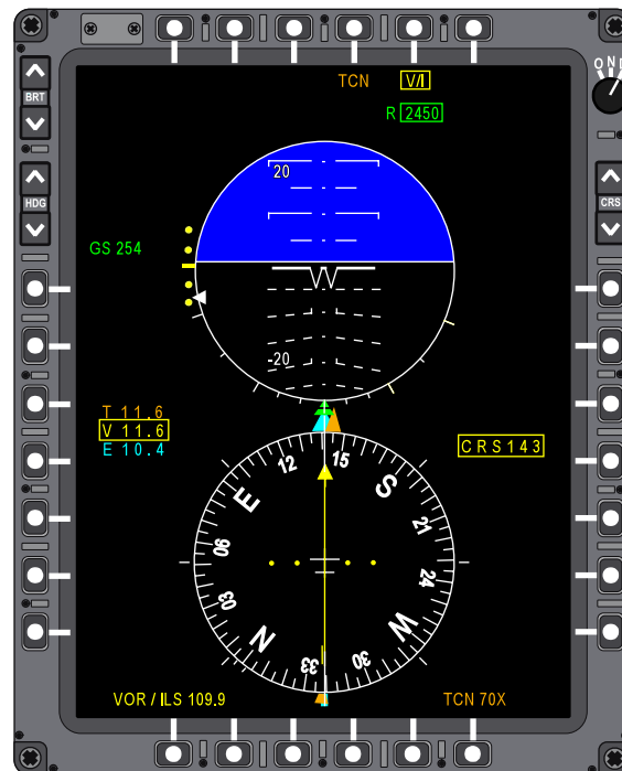
Figure 1-238. ILS Navigation Backup Operations
