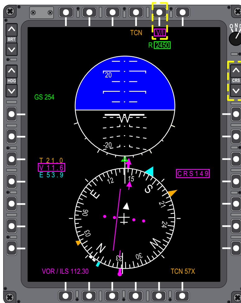
Figure 1-232. VOR Navigation Backup Operations
