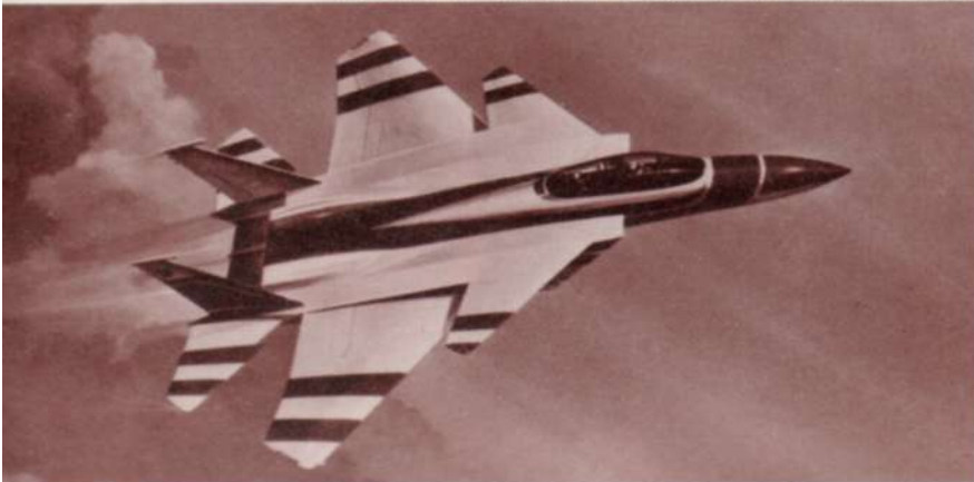
Advanced version of USAF F-15 with close-coupled canards.
