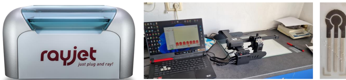
Picture 1 Photographs showing the Rayjet CO 2 laser engraver, the adapted system using a CNC diode laser engraver with an open source software and a picture of an electrode made with this machine.
