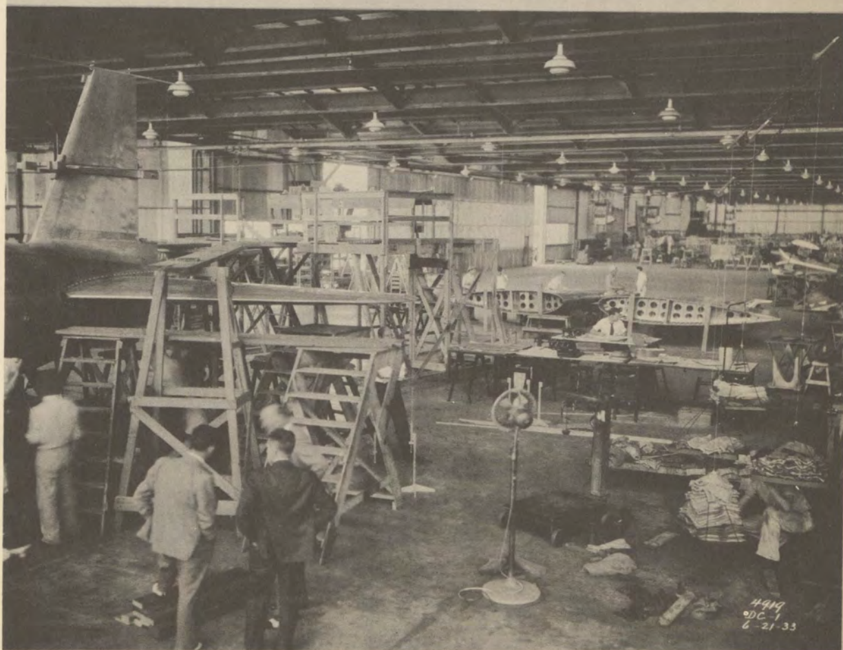
FUSELAGE TORSIONAL TEST. IN THIS TEST SIDE LOADS WERE APPLIED TO THE VERTICAL STABILIZER THROUGH A SYSTEM OF CABLES, PULLEYS AND WEIGHTS.
