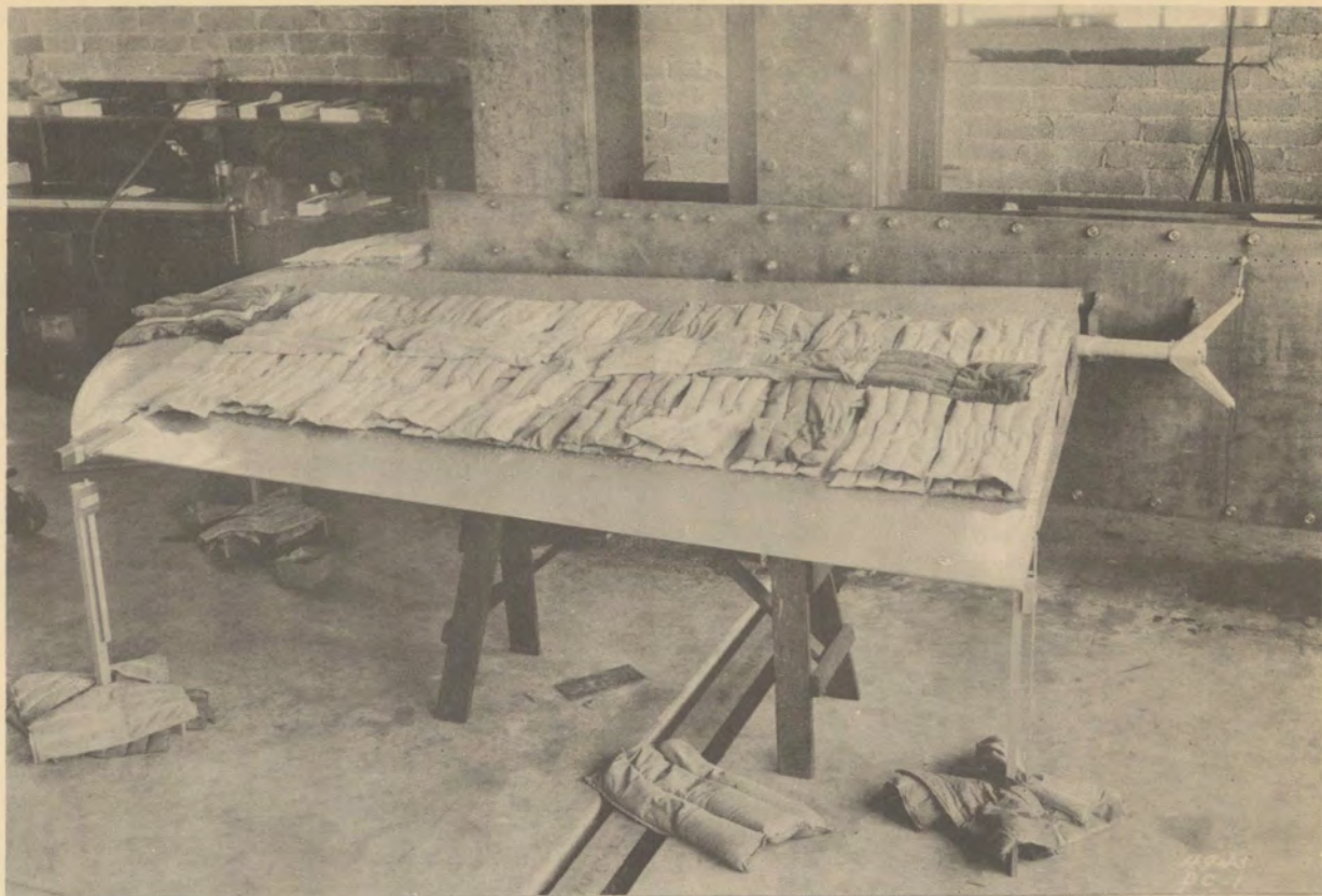
METAL COVERED RUDDER, STATIC TEST TO FULL DESIGN LOAD.
