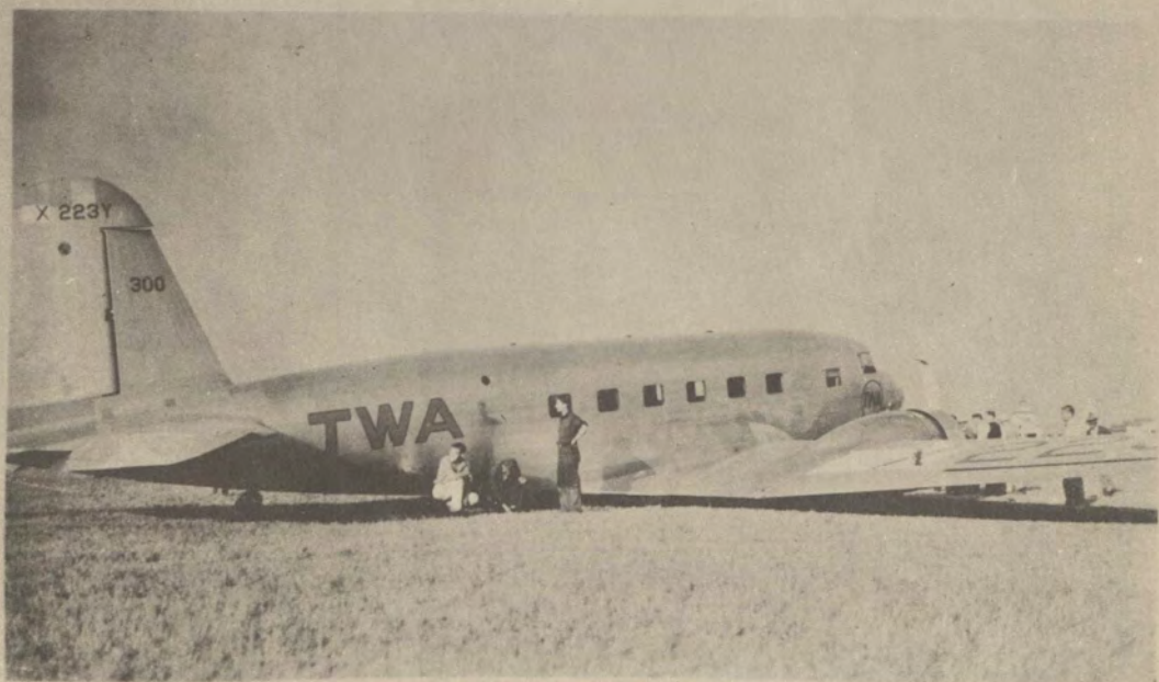
VIEW OF AIRPLANE AFTER LANDING WITH WHEELS RETRACTED. NEW PROPELLERS WERE INSTALLED AND THE AIRPLANE WAS FLOWN AWAY.
