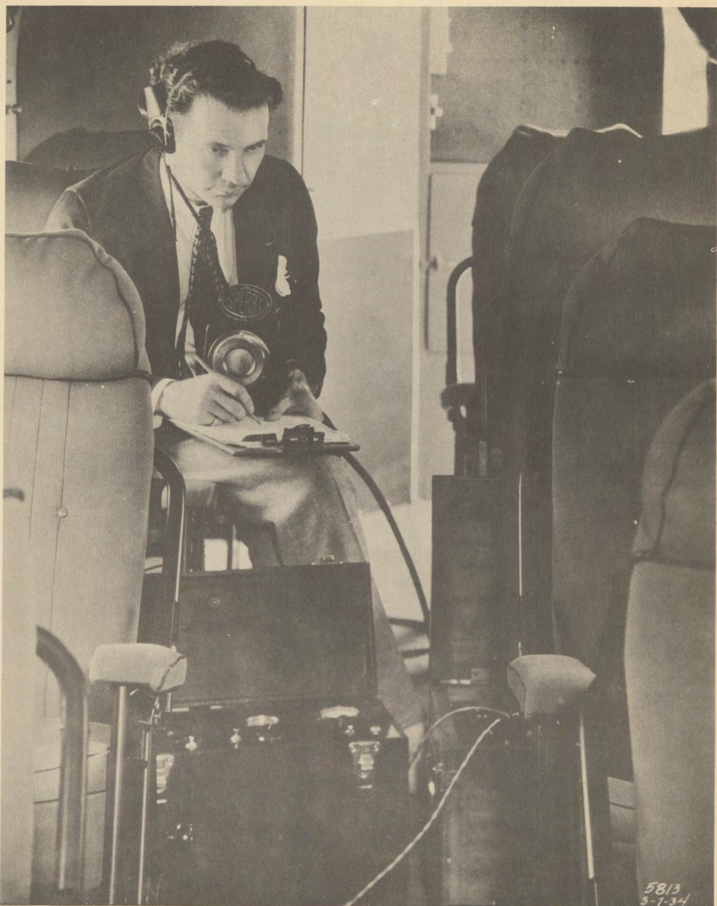
ACOUSTICAL ENGINEER MEASURING SOUND IN THE CABIN OF THE DOUGLAS TRANSPORT.
