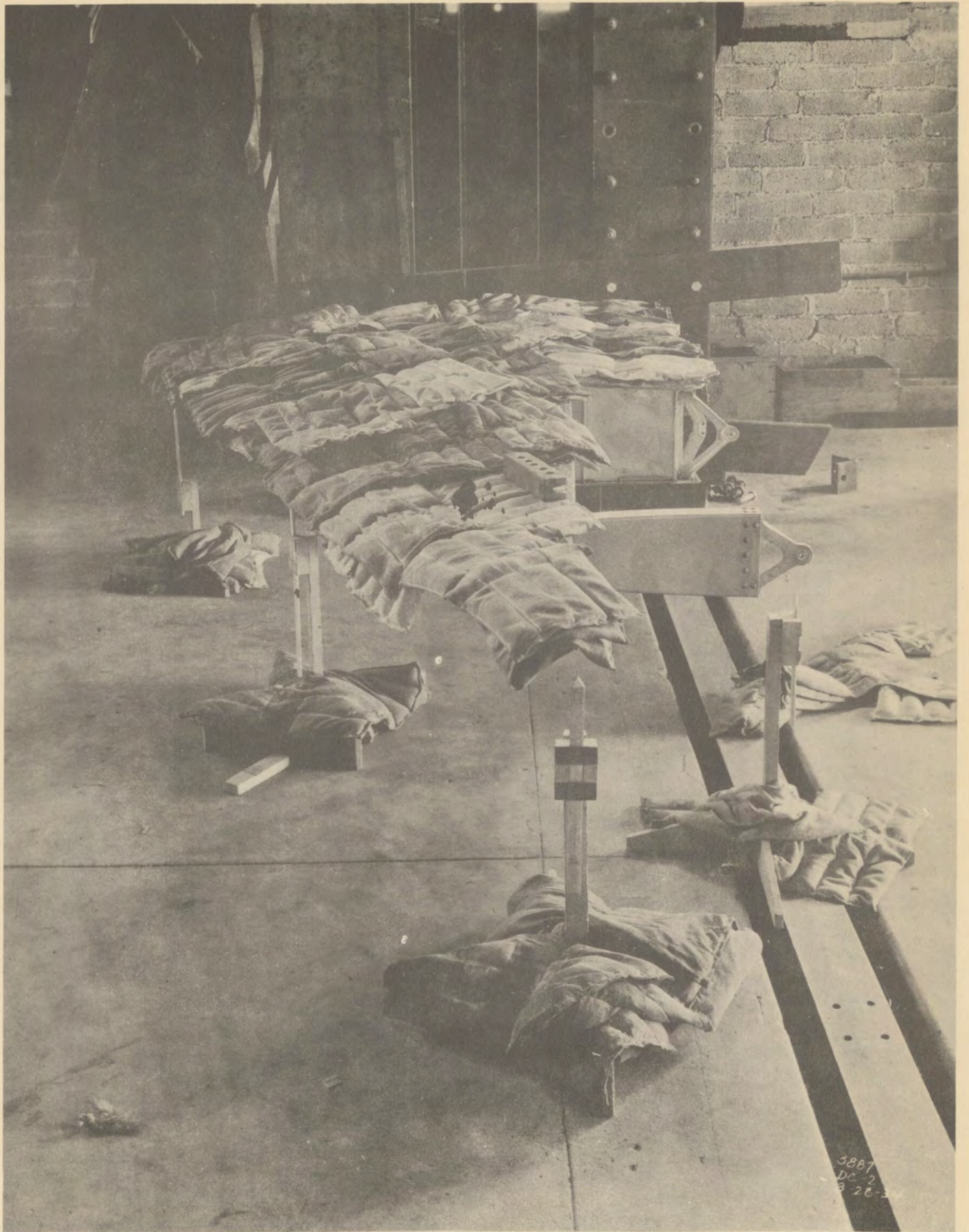
VERTICAL STABILIZER UNDER FULL DESIGN LOAD.
