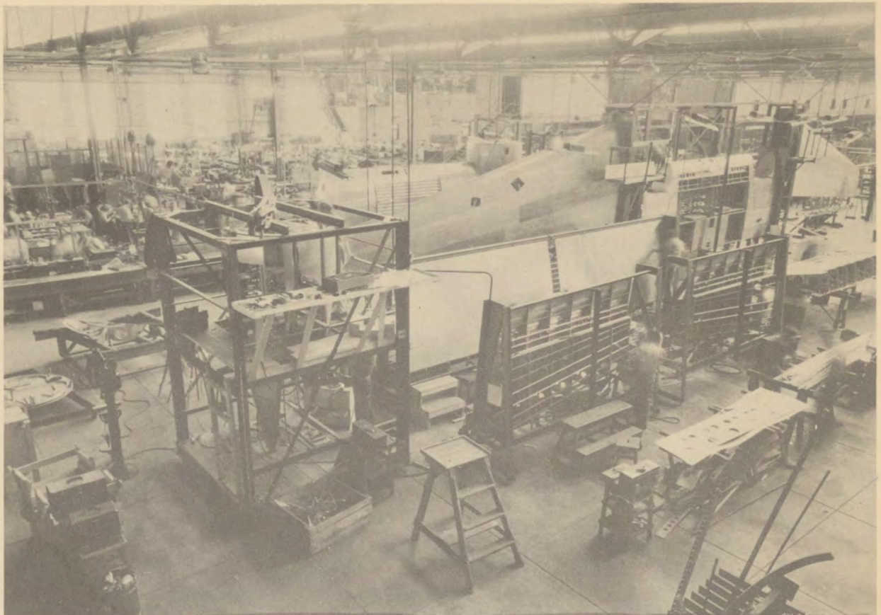
A PORTION OF THE WING DEPARTMENT AT THE DOUGLAS FACTORY. IN THE LEFT FOREGROUND IS AN ENGINE NACELLE ASSEMBLY JIG AND IN THE RIGHT FOREGROUND JIGS FOR ASSEMBLY OF WING TRAILING EDGE SECTIONS, BEHIND THESE A JIG FOR ASSEMBLY OF CENTER WING PANELS WITH OUTER WING PANEL JIGS AT EITHER SIDE.
