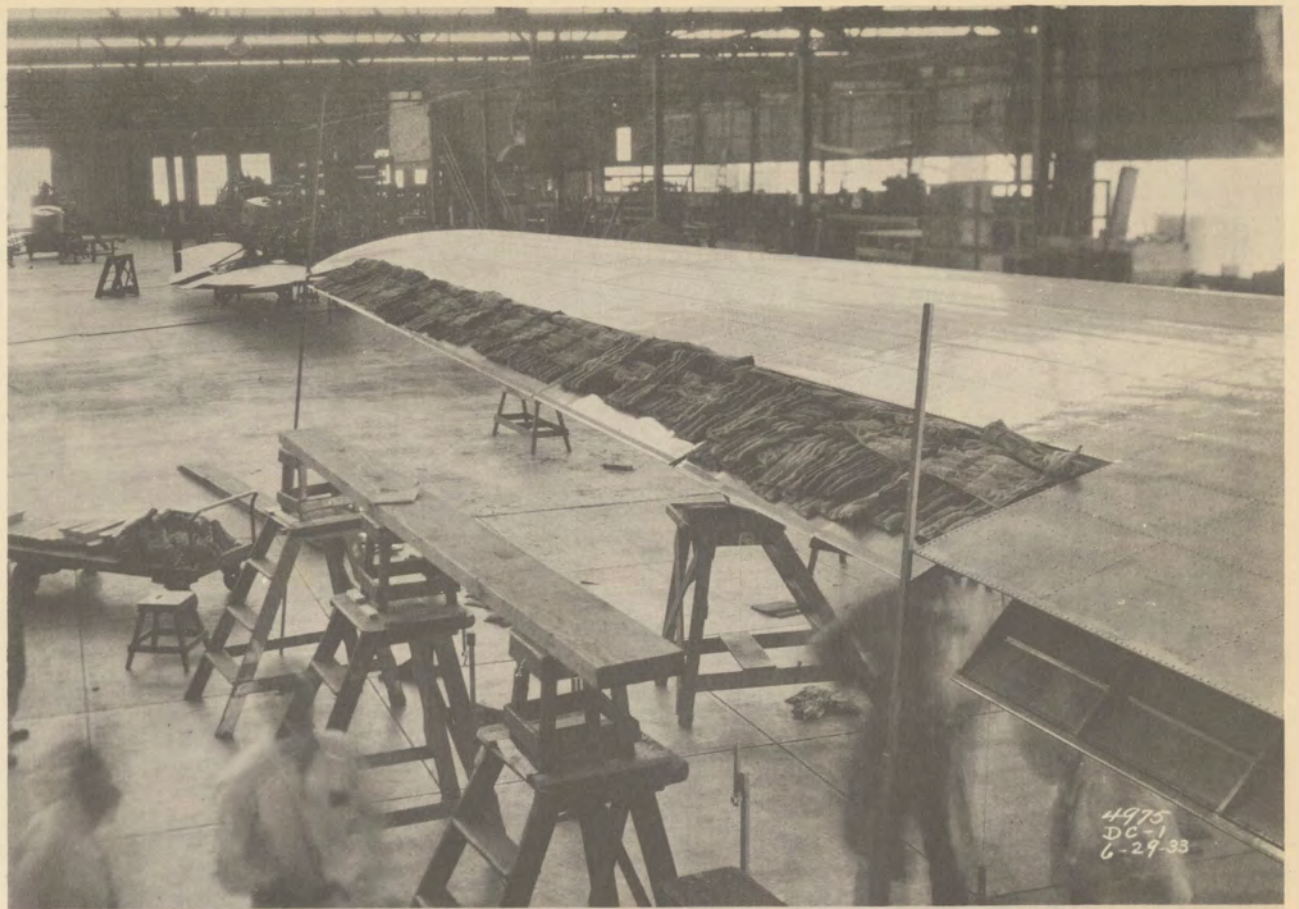
AILERON UNDER FULL STATIC LOAD.
