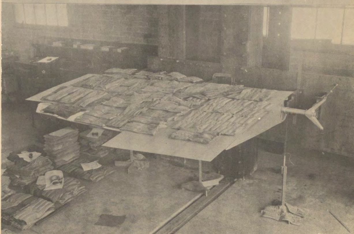
FABRIC COVERED RUDDER STATIC TEST TO FULL DESIGN LOAD.
