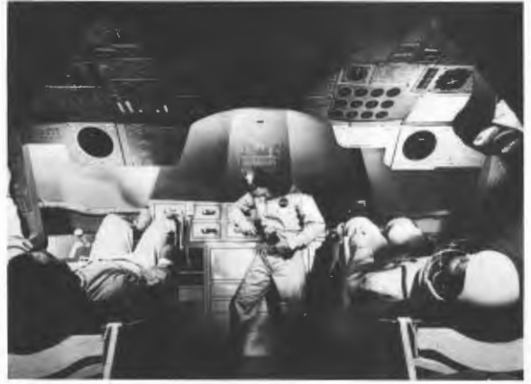
Interior of a partial full-scale mockup of the Apollo command module, above. In flight, the center couch would be removed (as shown), giving better access to the instrument panel and lower equipment bay. At left, left to right, astronauts Scott Carpenter, John Glenn, and Walter Schirra in 1963 inspect a full-scale mockup of the Apollo CM, designed for three men.
