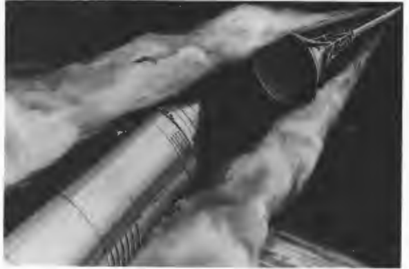
Full-scale model of the command module, above: the strake aerodynamic devices may be seen at either side of the spacecraft just above the aft heatshield. On the drawing of the launch escape system at upper right, the canard aerodynamic devices are near the top of the escape tower. Jettison of the launch escape system (right), after successful launch, also pulls away the boost protective cover that protects the windows from flame and soot.
