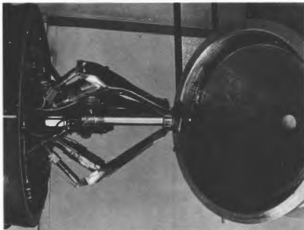
Spacecraft docking devices: the command module probe and docking ring at left; the lunar module drogue at right.
