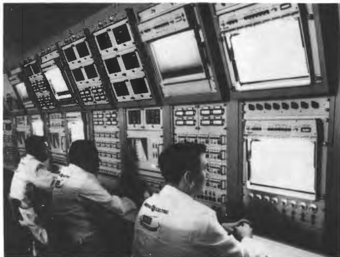
General Electric employees monitor activities of a spacecraft test in the automatic-checkout-equipment spacecraft control room in 1965.
