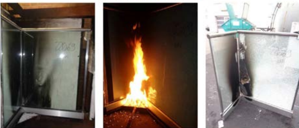
Fire testing before and after
