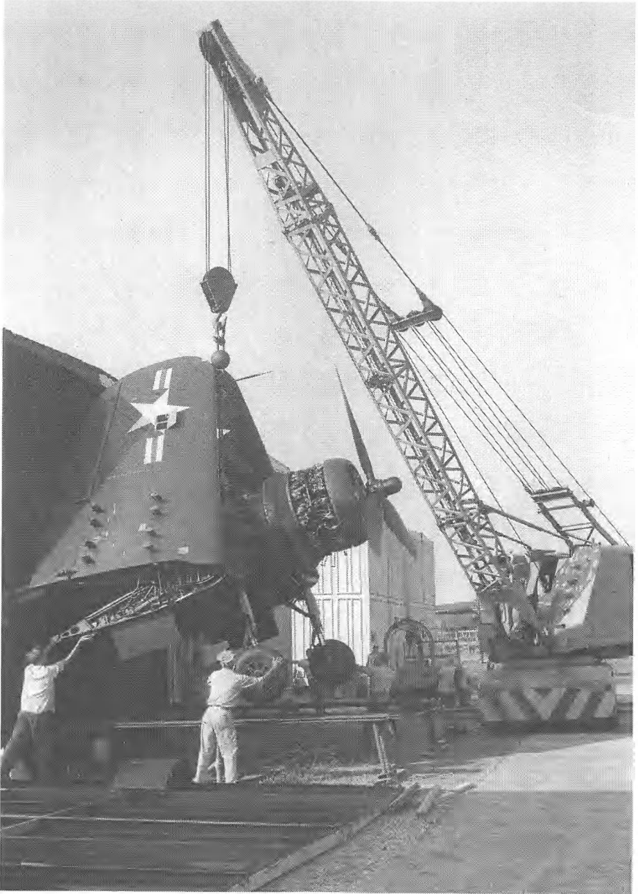
Repositioning F4U Corsair with crane after final assembly. Image source/ credit: Courtesy of the Igor I. Sikorsky Historical Archives, Inc.
