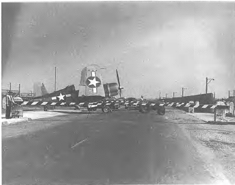
F4U being towed across Main Street from the final assembly area to the flight test hangars at Bridgeport Airport. Image source/ credit: Courtesy of the Igor I. Sikorsky Historical Archives, Inc.
