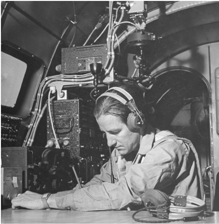
The radio operator was sat opposite the flight engineer, and from his station he operated a wide selection of communications equipment. Aside from the three SCR-type sets fitted in the aircraft, the radio operator also controlled the Type RC-21-T2 that could be used to call a crew member via any of the 24 interphone jack boxes located at each station within the XB-19. (Peter Stackpole/The LIFE Picture Collection via Getty Images)
