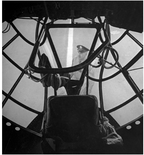
The bombardier's position was located below and aft of the nose turret, being accessible from the main cabin. This photograph of the position was taken looking down the stairs from the bridge deck, with the bomb aimer's seat folded flat. There are no records or photographs indicating that the top-secret Norden Type M-1 Bombsight was ever mounted in the aircraft. (Peter Stackpole/The LIFE Picture Collection via Getty Images)
