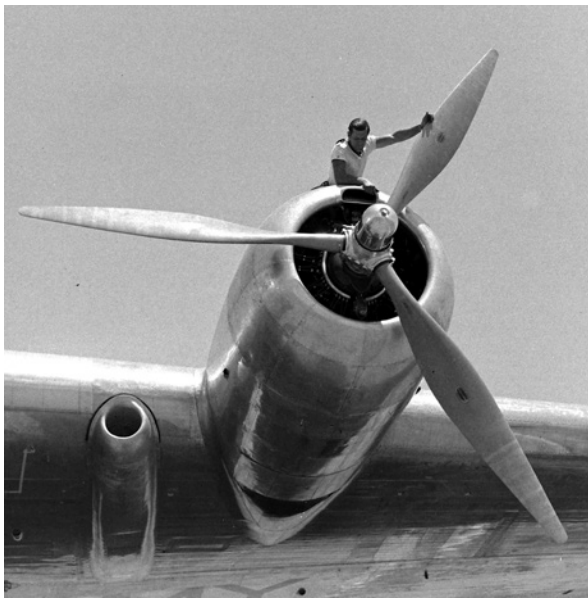
The four 700lb Hamilton-Standard 17ft-diameter, constant-speed, full-feathering, Hydromatic propellers were the largest to equip any aircraft at the time, dwarfing the DC-3's 11.3ft-diameter propellers. Later, the B-29's R-3350s swung a 16.7ft-diameter propeller. (Peter Stackpole/The LIFE Picture Collection via Getty Images)
