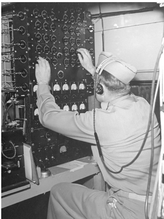
This bank of instrumentation was used to monitor the extensive network of strain gauges that were installed throughout the XB-19. (Peter Stackpole/The LIFE Picture Collection via Getty Images)
