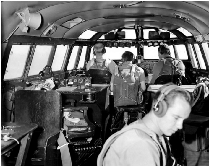
The bridge deck, with its many windows, is shown here with the pilot (Umstead), co-pilot (Bunker) and the flight engineer (Warren Dickerson) directly behind them – they are all wearing their parachutes. The radio operator is seen in the right foreground. The empty seat behind the pilot was usually occupied by the navigator, with the one opposite it assigned to the aircraft commander. (Author's Collection)
