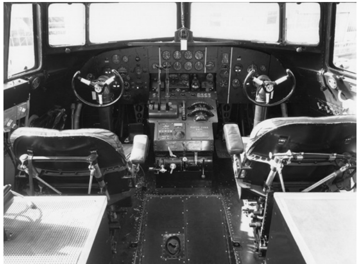
An unobstructed view of the forward cockpit. The flight instruments were mounted on three panels, with the left panel for the pilot, the right panel for the co-pilot, and the center panel visible to both. Both wheel-and-column controls are adorned with Douglas' "First Around the World" company logo on their center hubs. (Philip Jarrett Collection)
