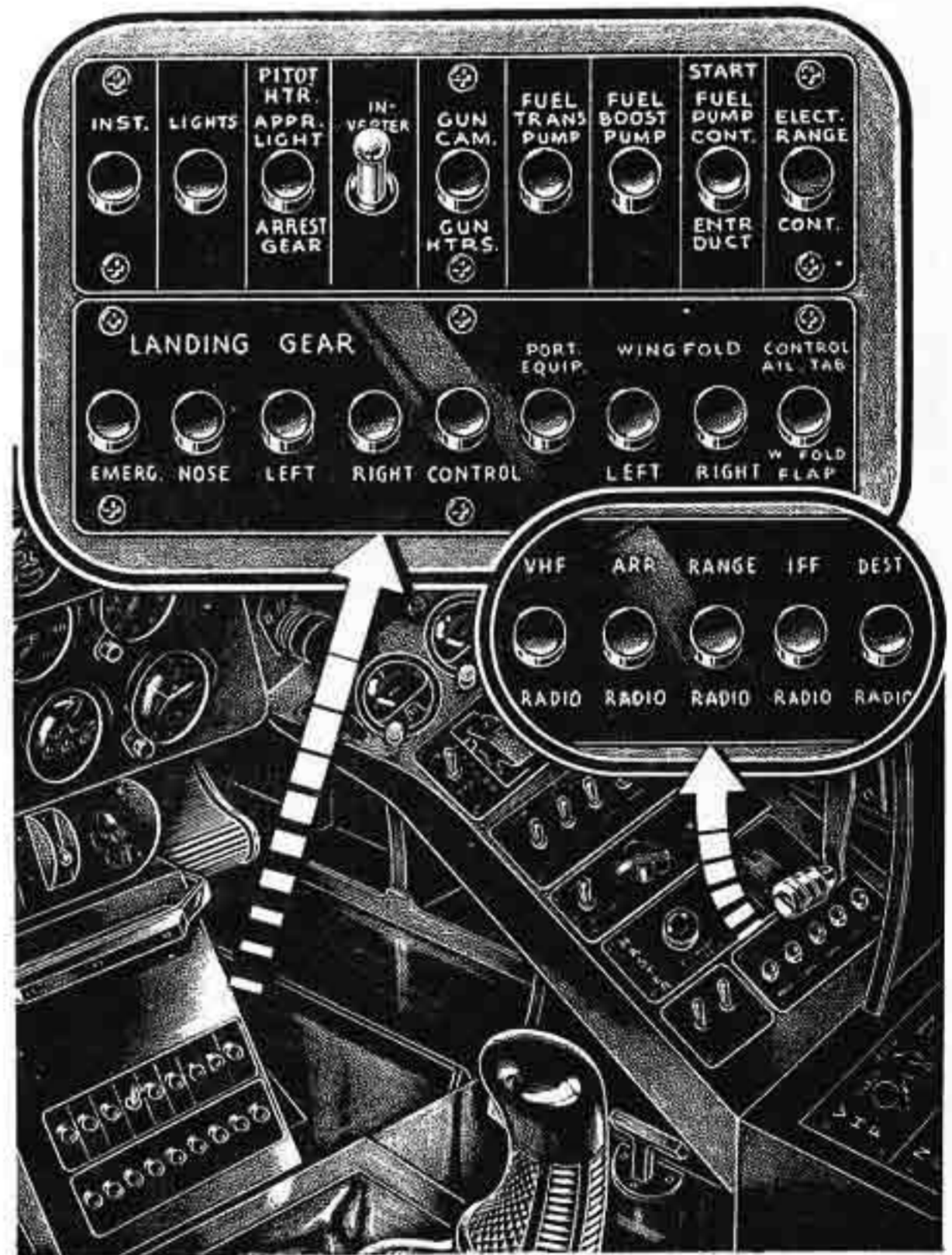
Figure 1-18. Main Distribution Panel
