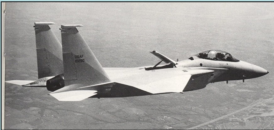
1 st FLIGHT CONFIG (Buffet OK at 35 deg, not enough drag)
