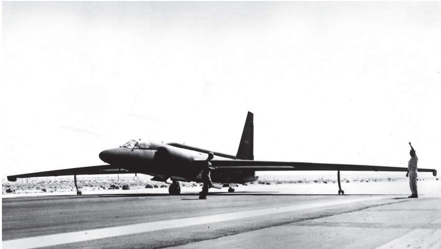
The Lockheed U-2, with an 80-foot wingspan, flew at over 70,000 feet and gathered not only information on Soviet strategic capabilities, but also data required in crisis situations. (Central Intelligence Agency)
