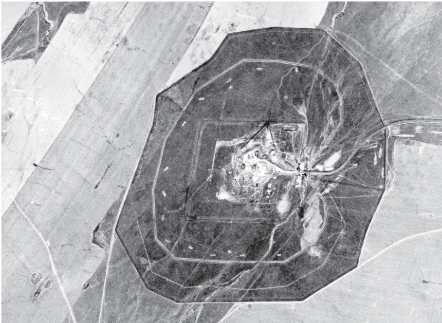
The Soviet penchant for horizontal security is typified by the five fences that surround an SS-5 intermediate-range missile site. This type of construction was always a dead giveaway and made the job of locating Soviet strategic installations much easier for the photo interpreter. (Central Intelligence Agency)
