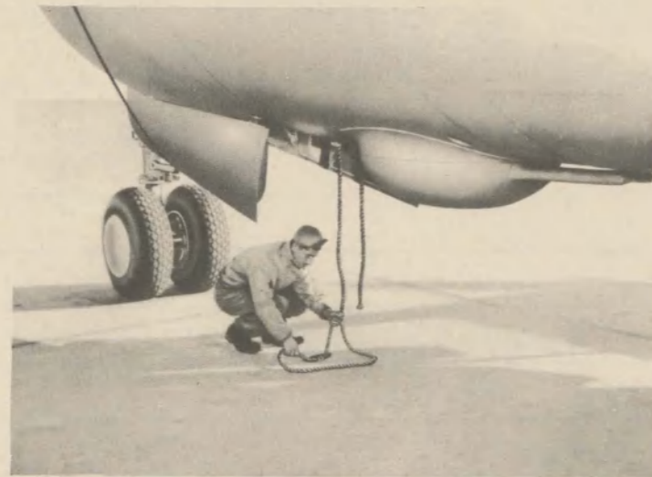
C ATTACHMENT TO THE NOSE WHEEL TIE DOWN FITTING AND ANCHORING TO THE GROUND
