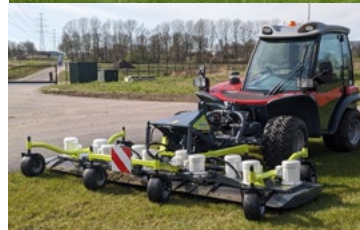
Eco Clipper FM343 343 cm mowing width
